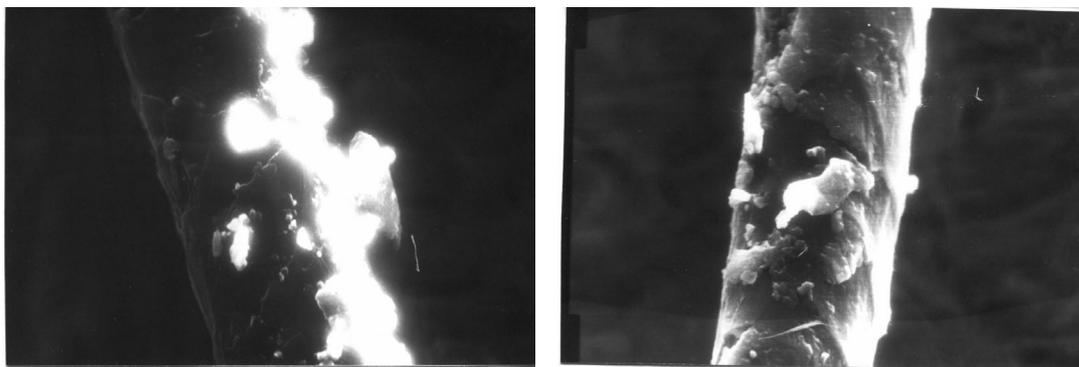
Fig. 2 – SEM images (x 1.800) of the wool fibre before (a) and after thermal treatment with biocatalyst I<sub>2</sub> at pH=7.5 (b).
