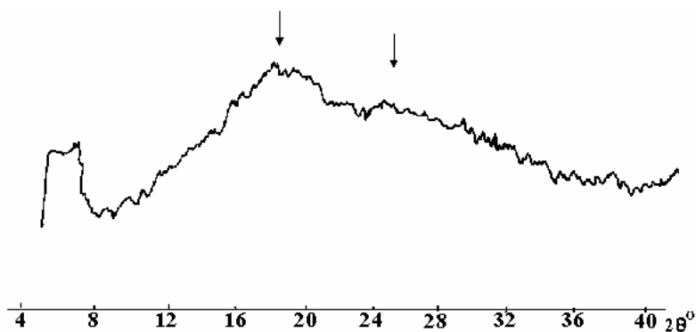
Fig. 2 – X-Ray diffraction diagram of poly[N-(3-acetoxy-4-carboxy-phenyl)-maleimide].
