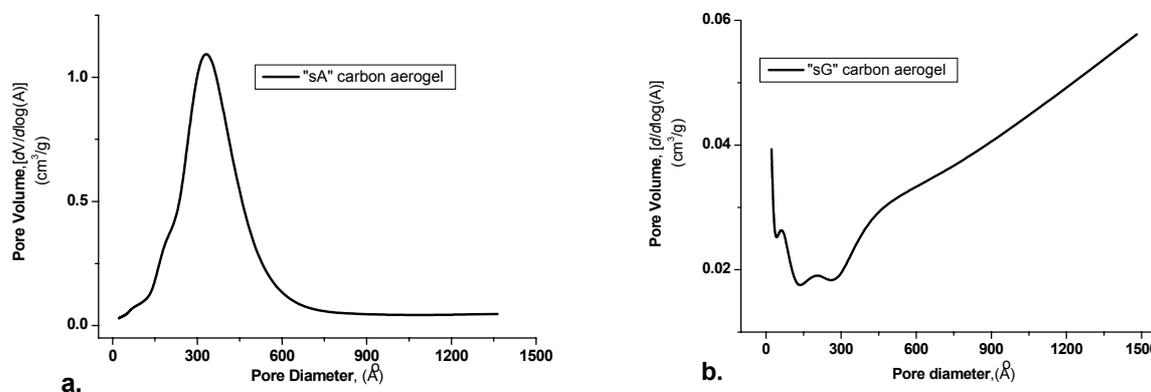
Fig. 2 – Pore size distribution of the “sA”(a) and “sG”(b) carbon aerogels.
