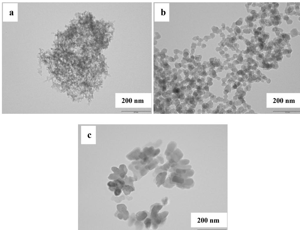
Fig. 4 – TEM images of the “sC” (a), “sH” (b), “sI” (c) carbon aerogels samples.
