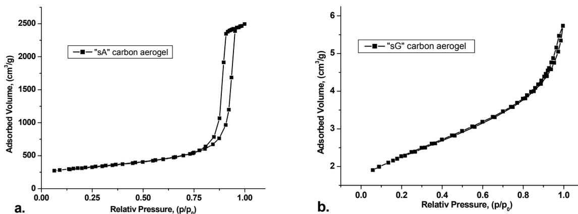
Fig. 1 – Adsorption-desorption isotherms of N<sub>2</sub> on the “sA”(a) and “sG”(b) carbon aerogels.
