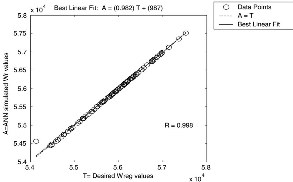
Fig. 3 – Results of the regression analysis between the ANN model response and the corresponding targets, for the catalyst inventory in the reactor variable  $W_r$  (testing set of data).
