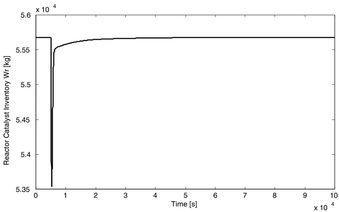
Fig. 8 – ANN based MPC of the catalyst inventory  $W_r$  in the reactor, in the presence of  $\Delta P_{fac}$  disturbance.
