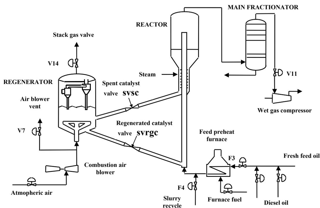
Fig. 1 – Schematic representation of the UOP Fluid Catalytic Cracking Unit.
