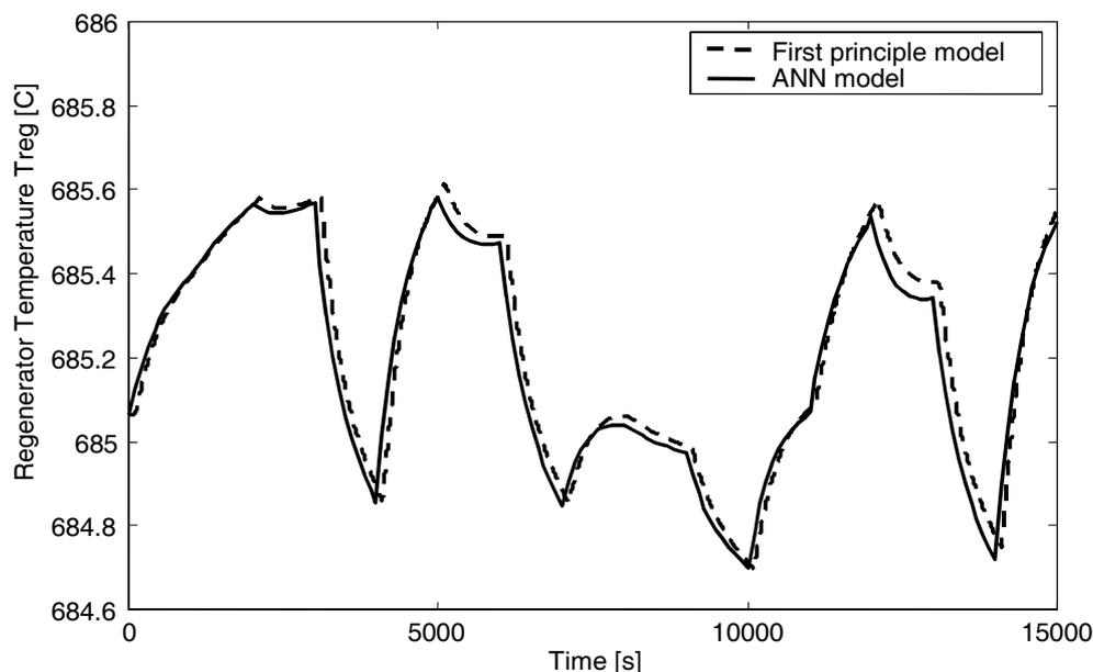
Fig. 5 – Comparative simulation results of ANN and first principle models, presenting the regenerator temperature simulated (target),  $T_{reg}$ .
