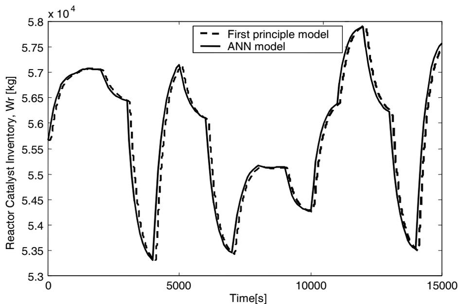
Fig. 4 – Comparative simulation results of ANN and first principle models, presenting the catalyst inventory simulated (target) variable,  $W_r$ .
