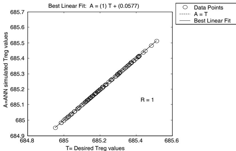
Fig. 2 – Results of the regression analysis between the ANN model response and the corresponding targets, for the temperature of the regenerator bed variable  $T_{reg}$  (testing set of data).
