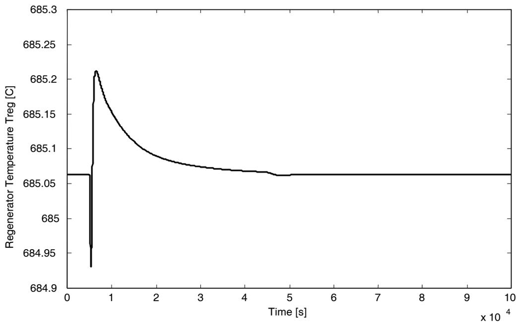
Fig. 9 – ANN based MPC of the regenerator temperature  $T_{reg}$  in the presence of  $\Delta P_{frac}$  disturbance.
