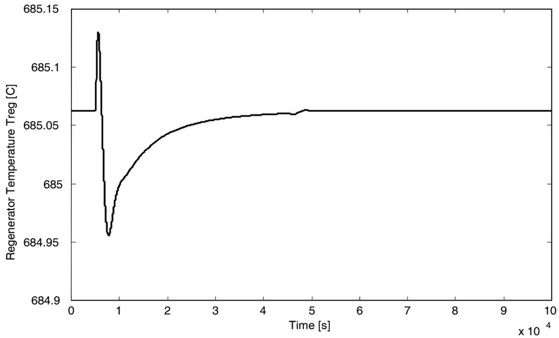
Fig. 7 – ANN based MPC of the regenerator temperature  $T_{reg}$  in the presence of the intensity of catalyst coking disturbance.
