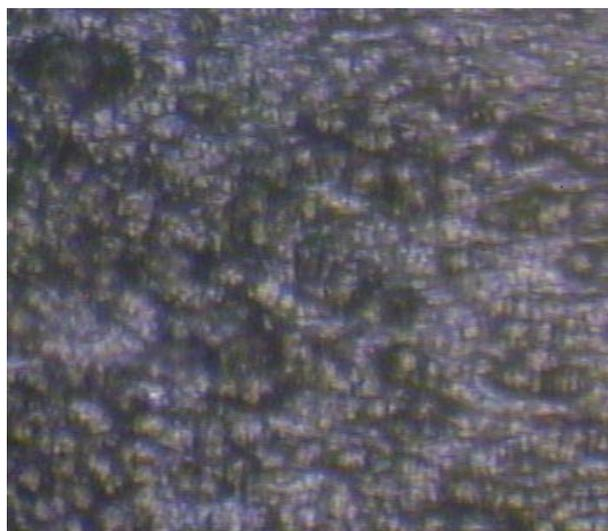
Fig. 4 – Micrography of PPY film electrodeposited on aluminum surface after 25 cycles.
