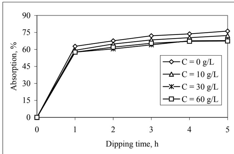
Fig. 4 – Water absorption of EW-SA samples for different SA concentration levels.
