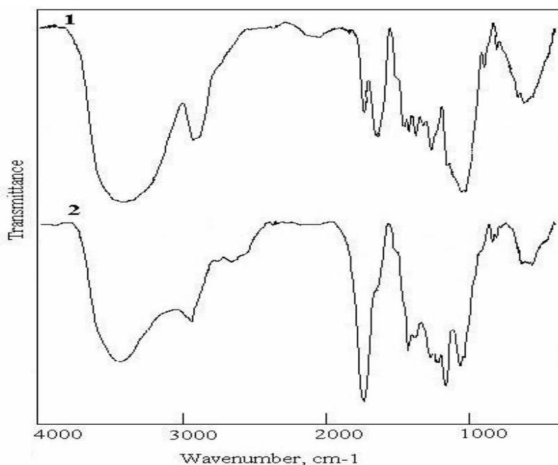
Fig. 1 – FTIR spectra for fir wood flour: 1.EWF; 2. EWF-SA.
