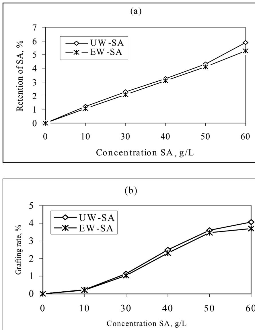
Fig. 2 – Variation of retention (a) and grafting rate (b) with SA concentration value (dipping time: 7 min).
