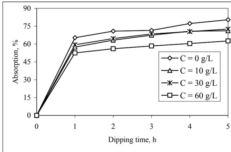
Fig. 3 – Water absorption of UW-SA samples for different SA concentration levels.
