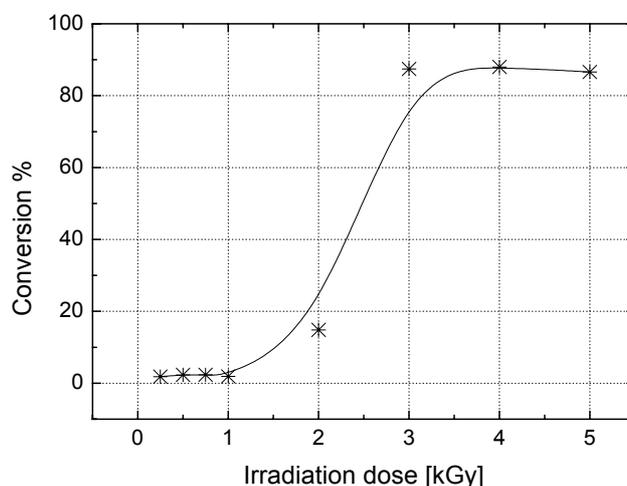
Fig. 2 – The yield of polymerization of methyl acrylate versus the irradiation dose for the methyl acrylate/ gypsum composites.
