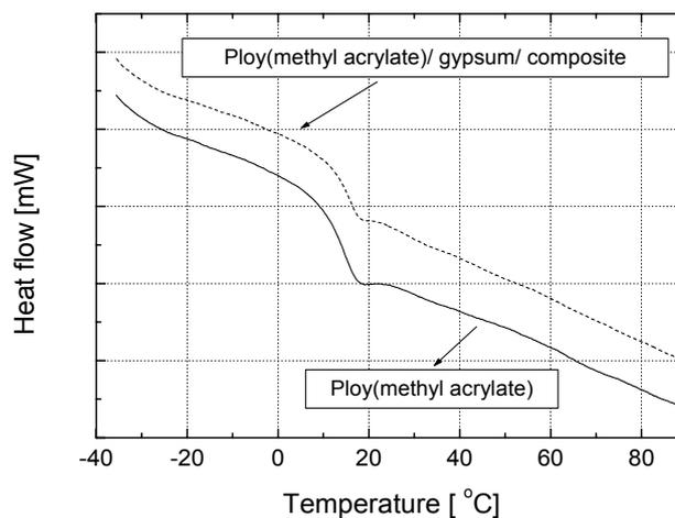
Fig. 4 – DSC spectra for pure poly (methyl acrylate) and poly (methyl acrylate)/ gypsum/ composite irradiated at 15 kGy.
