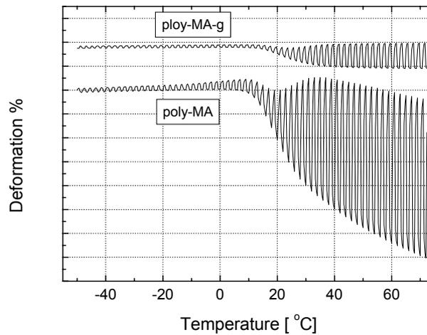
Fig. 3 – TMA spectrum with alternated force of 0.2 N for poly (methyl acrylate)/ gypsum/ composite irradiated at 5 kGy.
