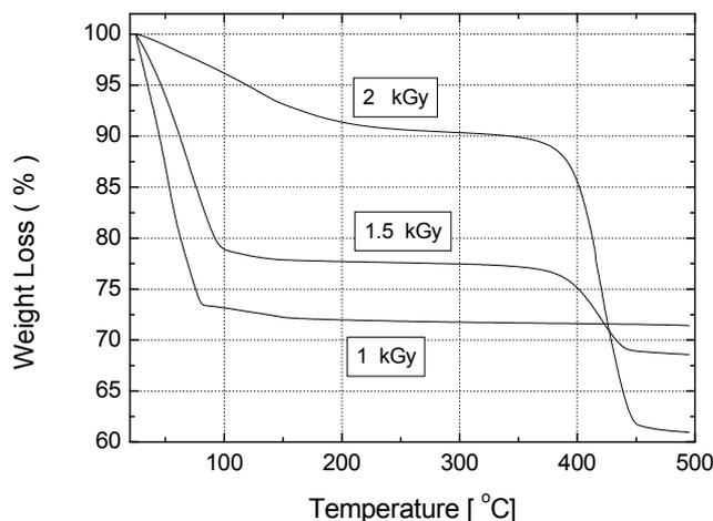
Fig. 1 – TGA thermograms of methyl acrylate/ gypsum/ composites for different preparation doses.
