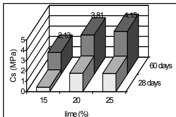
Fig. 6 – The influence of lime content on the compressive strength developed by the binders based on fly ash (water/binder=0.64).
