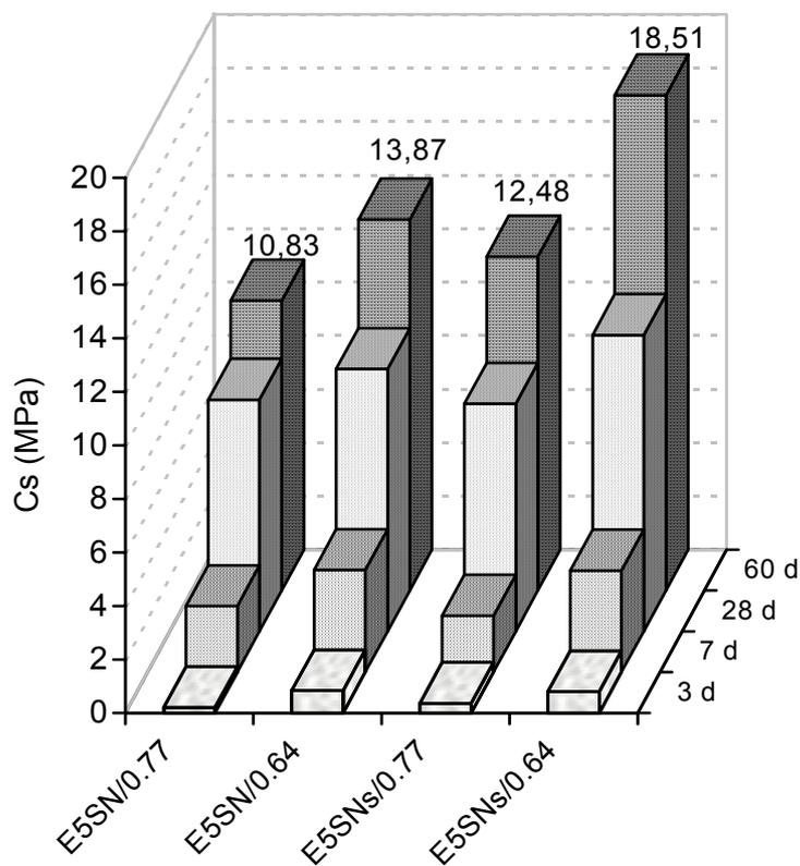
Fig. 8 – Compressive strength for the binders: **E5SN** - fly ash+ 20% lime + 5% sodium silicate +5% NaOH with w/b=0.77 and 0.64 and **E5SNs** - fly ash+ 20% lime + 5% sodium silicate + 4.2% Na<sub>2</sub>SO<sub>4</sub> with w/b=0.77 and 0.64.
