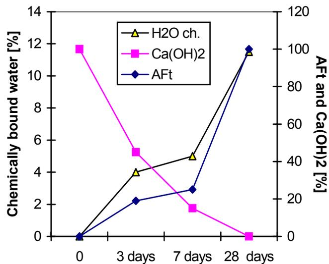
Fig. 4 – Hydrates vs. time for mixture E5SNs. Chemically bound water and Ca(OH)<sub>2</sub> content was assessed by TG and ettringite (AE<sub>t</sub>) content by XRD.
