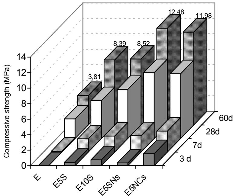
Fig. 7 – Compressive strength for the binders: **E** – fly ash+ 20% lime (w/b=0.64); **E5S** - fly ash+ 20% lime + 5% sodium silicate (w/b=0.77); **E10S** - fly ash+ 20% lime + 10% sodium silicate (w/b=0.84); **E5SNs** - fly ash+ 20% lime + 5% sodium silicate + 4.2% Na<sub>2</sub>SO<sub>4</sub> (w/b=0.77); **E5NCs** - fly ash+ 20% lime + 5% NaOH and 5% CaSO<sub>4</sub> (w/b=0.5).
