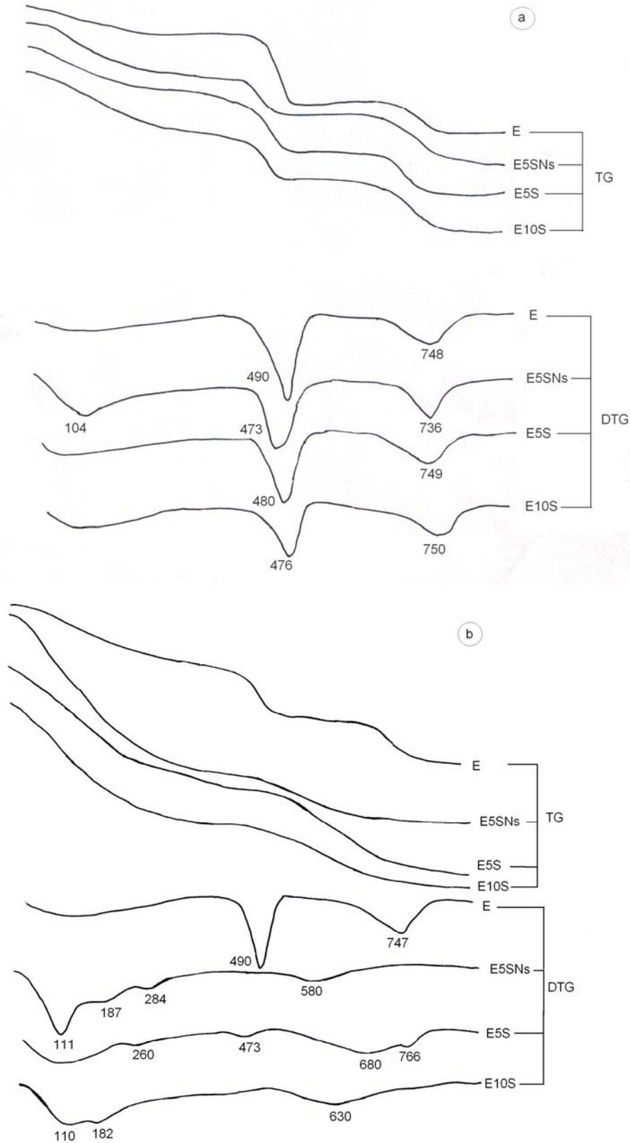
Fig. 2 – TG and DTG curves of the pastes cured for 3 days (a) and 28 days (b). **E** – fly ash+ 20% lime; **E5S** - fly ash+ 20% lime + 5% sodium silicate; **E10S** - fly ash+ 20% lime + 10% sodium silicate; **E5SNs** - fly ash+ 20% lime + 5% sodium silicate + 4.2% Na<sub>2</sub>SO<sub>4</sub>.
