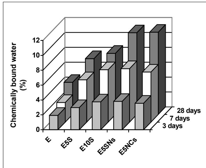
Fig. 5 – Chemically bound water in hydrates for the binders: E – fly ash+ 20% lime; E5S - fly ash+ 20% lime + 5% sodium silicate; E10S - fly ash+ 20% lime + 10% sodium silicate; E5SNs - fly ash+ 20% lime + 5% silicat de sodiu + 4.2% Na<sub>2</sub>SO<sub>4</sub>; E5NCs - fly ash+ 20% lime + 5% NaOH and 5% CaSO<sub>4</sub>.
