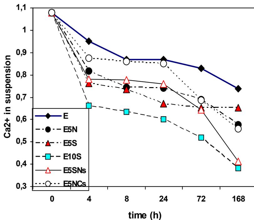
Fig. 1 –  $\text{Ca}^{2+}$  concentration in suspensions vs. time for: **E** – fly ash+ 20% lime; **E5S** - fly ash+ 20% lime + 5% sodium silicate; **E10S** - fly ash+ 20% lime + 10% sodium silicate; **E5N** - fly ash+ 20% lime + 5%NaOH; **E5SNs** - fly ash+ 20% lime + 5% sodium silicate + 4.2%  $\text{Na}_2\text{SO}_4$ ; **E5NCs** - fly ash+ 20% lime + 5% NaOH and 5%  $\text{CaSO}_4$ .
