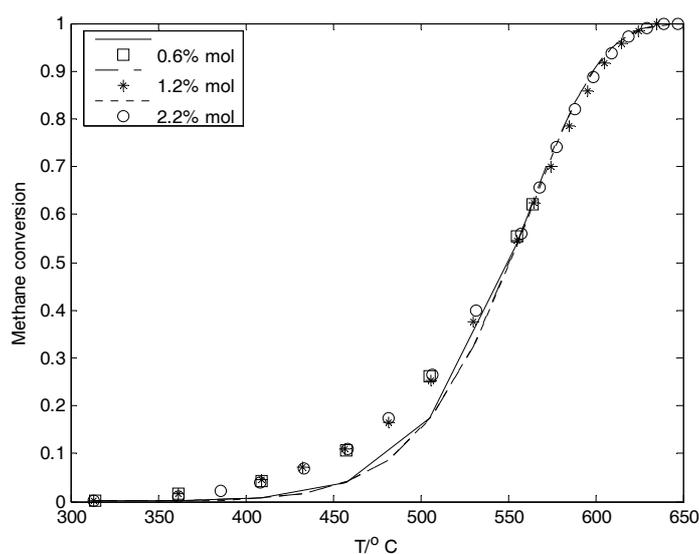
Fig. 7 – Combustion conversion-temperature curves for different methane feed concentrations (GHSV = 15000  $\text{cm}^3/(\text{g}_{\text{cat}}\cdot\text{h})$ , catalyst size 50-250 $\mu\text{m}$ ); the points represent measurements and the lines calculated values by kinetic model (14).
