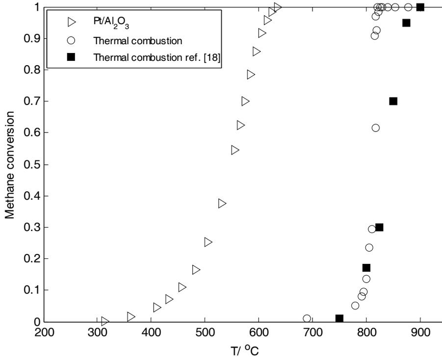
Fig. 3 – Methane conversion vs. temperature (1.2 mole % CH<sub>4</sub>, total flow rate 3000 cm<sup>3</sup>/h; 0.2 g catalyst; particle size 50-100 μm).
