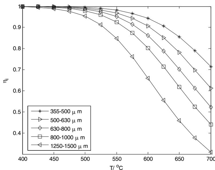
Fig. 8 – Calculated effectiveness factor (feed methane concentration 1.2 mol%; space velocity, 45000  $\text{cm}^3/(\text{g}_{\text{cat}} \text{h})$ ).
