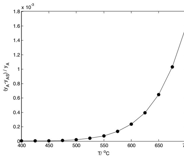
Fig. 4 – Temperature dependence of external concentration gradient.
