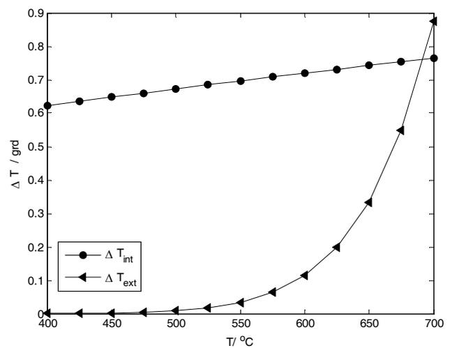
Fig. 5 – Temperature dependence of internal, respectively external temperature gradient.
