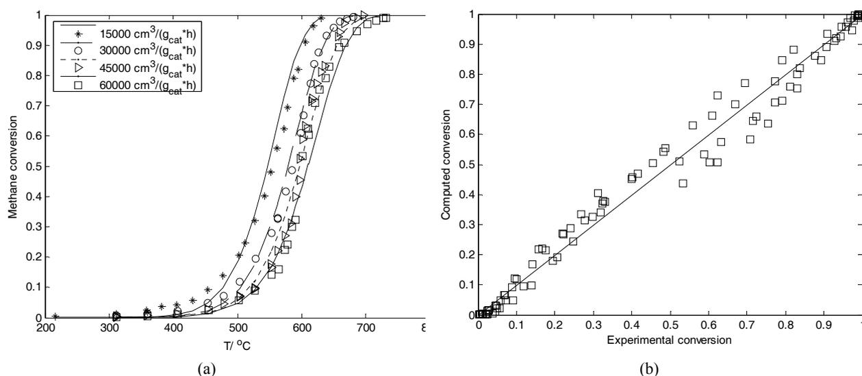
Fig. 6 – (a) Combustion conversion-temperature curves for different feed total flow rates (feed methane concentration 1.2 % mol, catalyst size 50-250 $\mu\text{m}$ ); the points represent measurements and the lines calculated values by kinetic model (14); (b) calculated versus experimental values of methane conversion (parity diagram).
