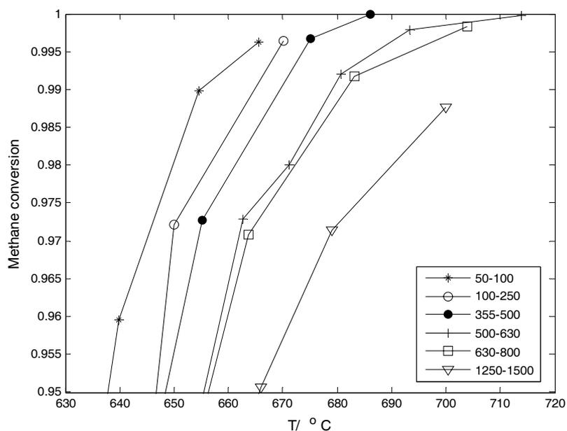
Fig. 1 – Experimental study of the internal diffusion influence for methane combustion over Pt/Al<sub>2</sub>O<sub>3</sub> catalyst.
