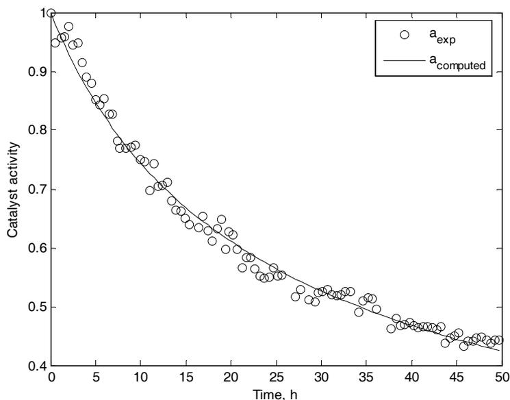
Fig. 10 – Catalyst activity as a function of on-stream time. The points represent experimental data and the line calculated values (1.2 mol % CH<sub>4</sub>; GHSV = 45000 cm<sup>3</sup>/(g<sub>cat</sub> h); T = 605°C).
