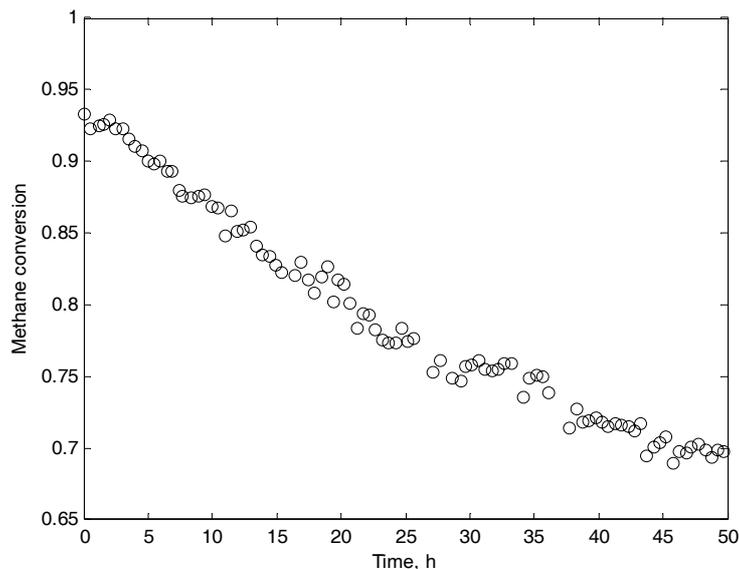
Fig. 9 – Methane conversion as a function of the time on stream (1.2 % CH<sub>4</sub> (mol), GHSV = 45000 cm<sup>3</sup>/(g<sub>cat</sub> h), T = 605°C).
