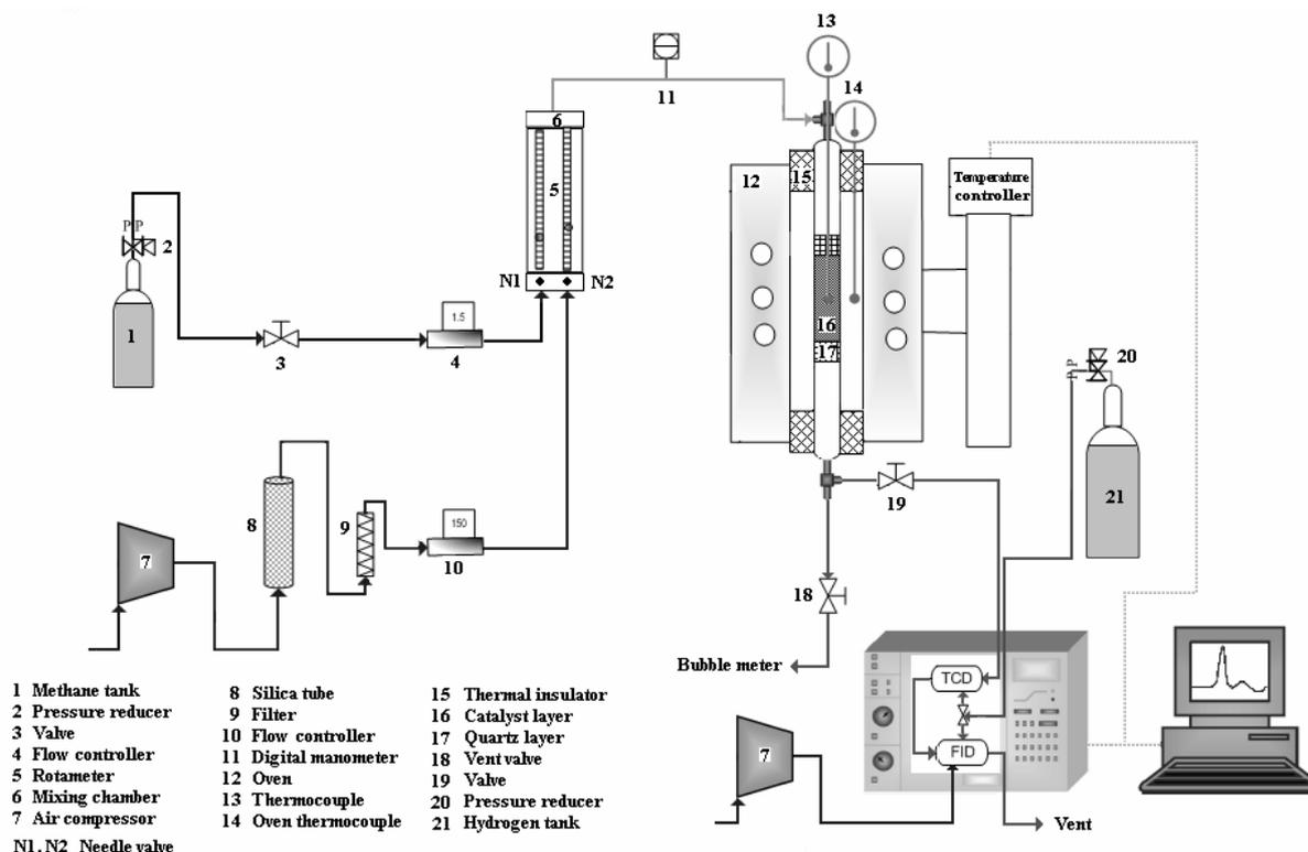
Fig. 2 – Schematic diagram of the experimental set-up for methane catalytic combustion.
