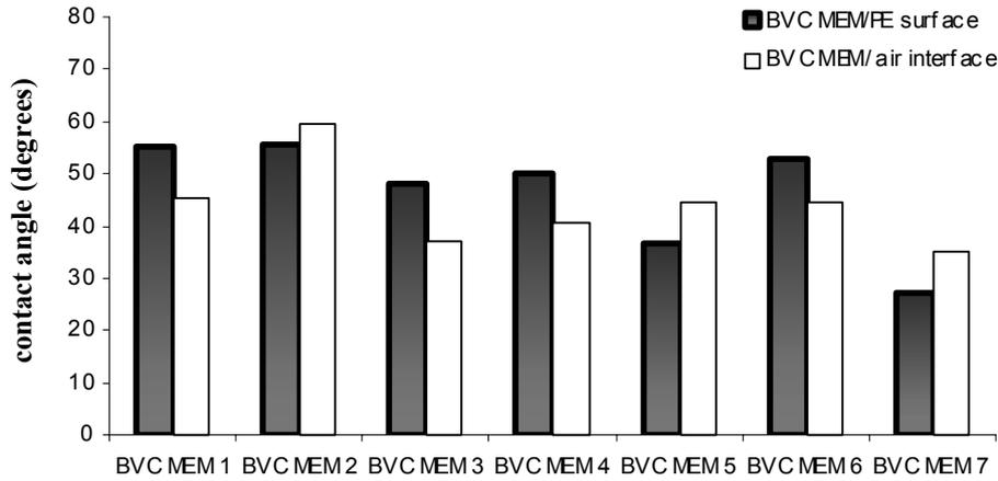
Fig. 2 – Contact angle  $\theta_{\text{DMSO}}$  on collagen-silicate membranes (BVC MEMs) at the air and PE interfaces at 20-21 °C.
