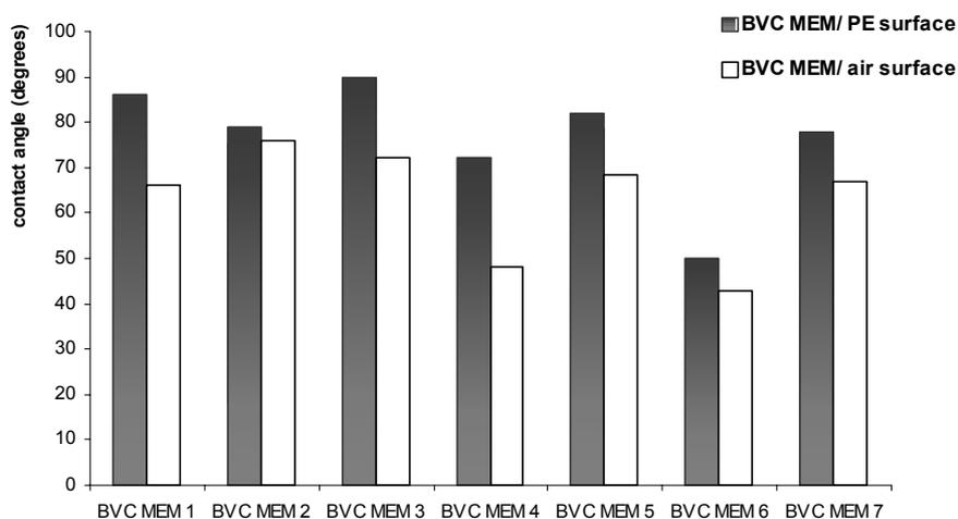
Fig. 1 – Water contact angle  $\theta_w$  on collagen-silicate membranes BVC MEMs/air and MEMs/PE at 20-21°C.
