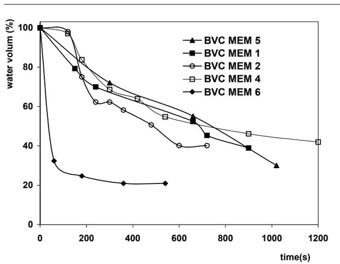
Fig. 3a – Variation of water droplets' volume (in percentages) with time for membranes BVC MEM 5,1,2,4,6 (only some experimental values are represented in this figure).
