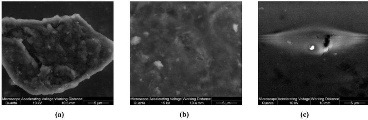
Fig. 4 – SEM images of BVC MEM 3 (a) BVC MEM 4 (b) and BVC MEM 6 (c) at accelerating voltage 10 kV working distance 10 mm; 5  $\mu\text{m}$  for (a,b,c).
