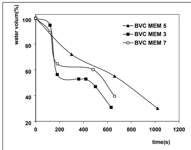
Fig. 3b – Variation of water droplets' volume (in percentages) with time for membranes BVC MEM 5,3,7 (only some experimental values are represented in this figure).
