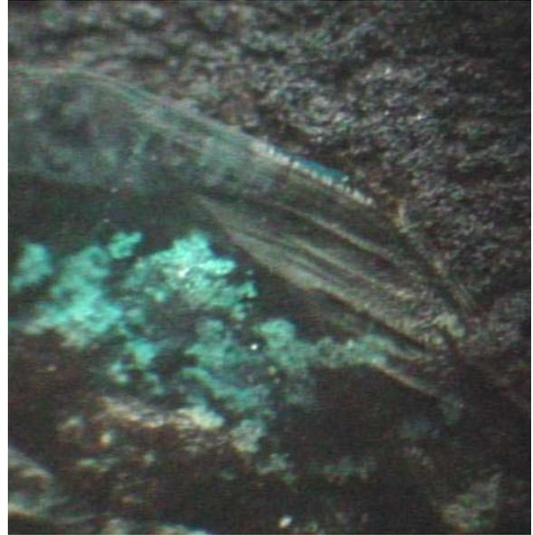
Fig. 2 – Images of the crystal formed on the cathodic surface (x25).
