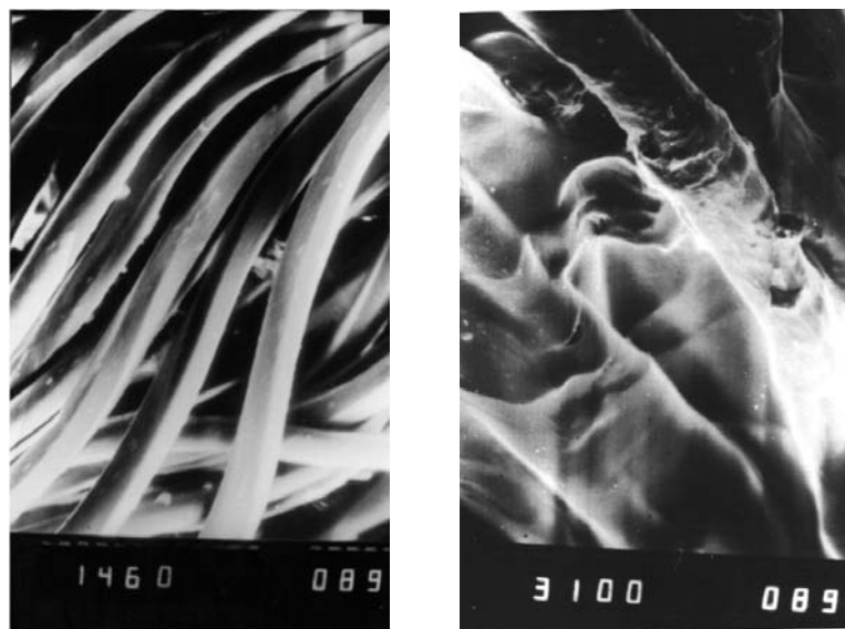
Fig. 5 – Scanning electron micrographs of untreated PA fabric (A) and PA/ Trox (B) (T#2).
