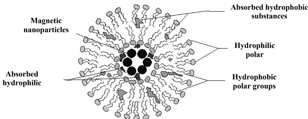
Fig. 2 – Structure of a magnetoliposome.
