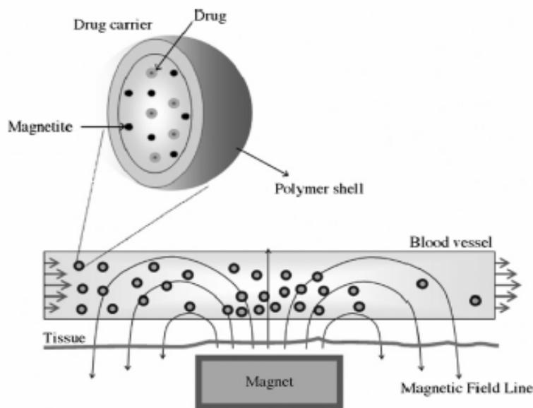
Fig. 5 – The schematic representation of drug magnetic vectoring: the magnetic carrier is directed to and releases the drug in the target area (Yang, 2006).<sup>10</sup>
