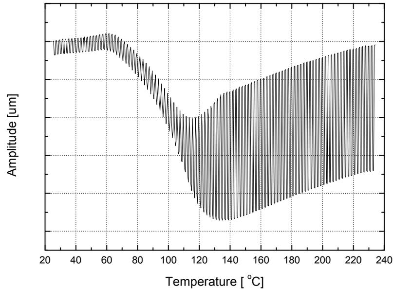
Fig. 4 – TMA thermogram with alternated force for polyester-styrene resin sample irradiated at 20 kGy.
