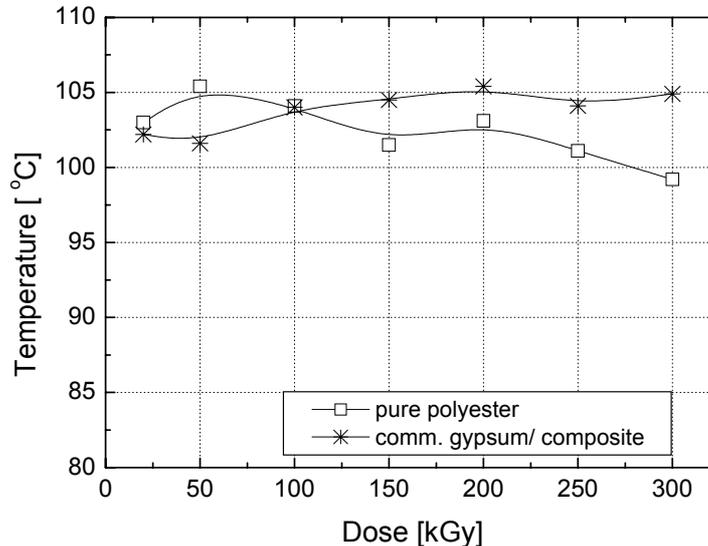
Fig. 5 – Glass transition temperatures of polyester-styrene resins and polyester-styrene resin/ gypsum/ composites versus the irradiation dose (TMA measurements with constant force).
