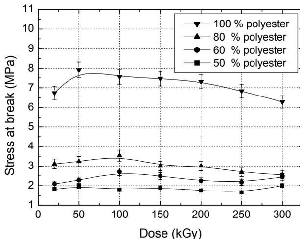
Fig. 1 – Stress at break (compression strength) of pure polyester-styrene resin and the prepared composites versus the irradiation dose (commercial gypsum).
