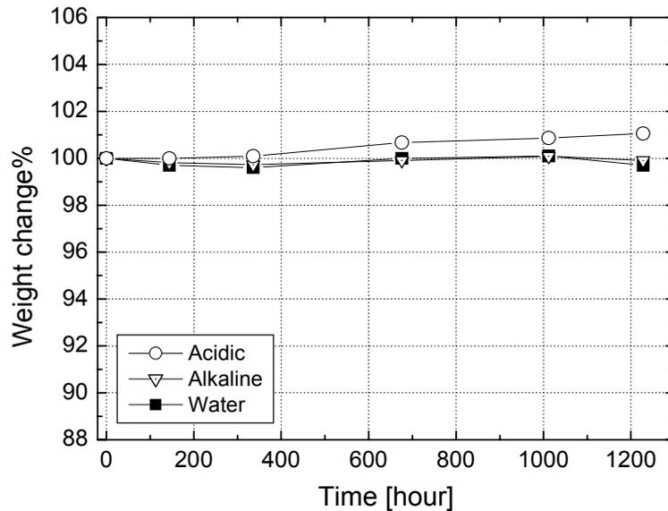
Fig. 6 – Water uptake of composites in solutions of different pH values, which are prepared at an irradiation dose of 20 kGy.
