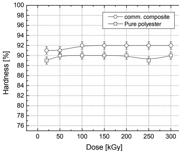
Fig. 2 – The hardness of pure polyester-styrene resin and the prepared composites versus the irradiation dose.
