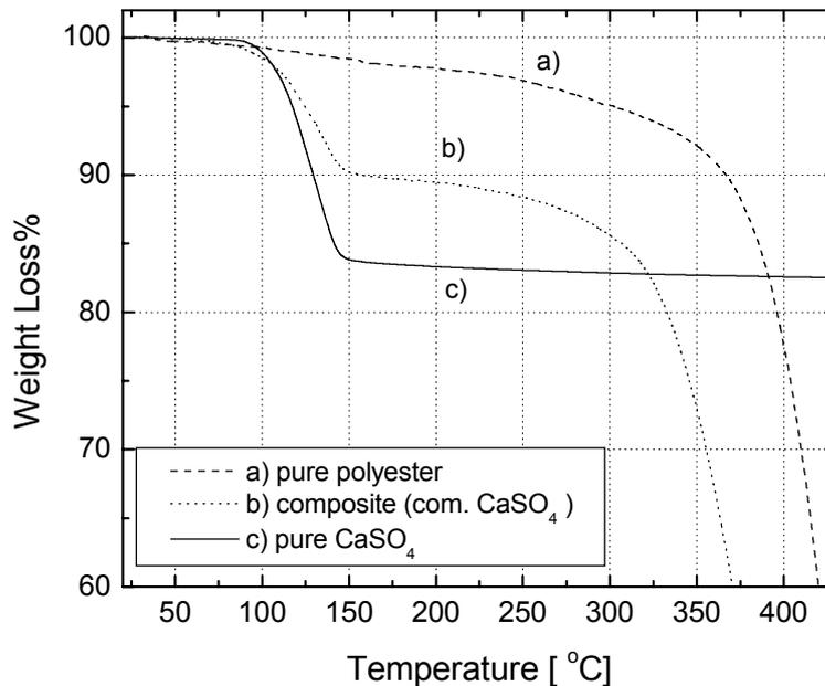
Fig. 3 – TGA thermograms of polyester-styrene resin and polyester-styrene resin/ gypsum/ composite in presence of nitrogen for samples irradiated at 20 kGy.
