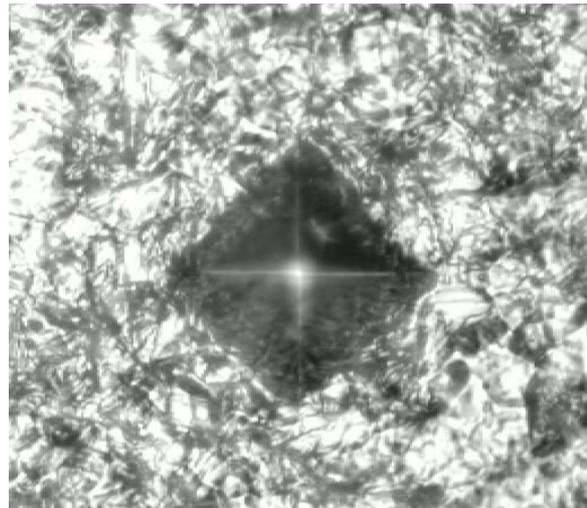
Fig. 5 – Photo of a hardness measurement for a sample of nickel deposited on a copper substrate from a Watts bath without additive, at -1000 mV potential and 65°C temperature (Shimadzu HMV, 400X optic magnitude).
