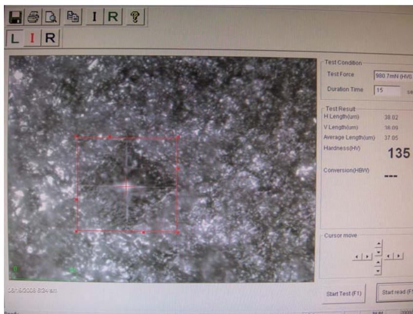
Fig. 3 – Measurement of an imprint of a sample of nickel electrodeposited from a Watts bath with addition of PVP at -1000 mV, 65°C temperature, and 15 minutes time. Applied force 0.1N (Shimadzu HMV).
