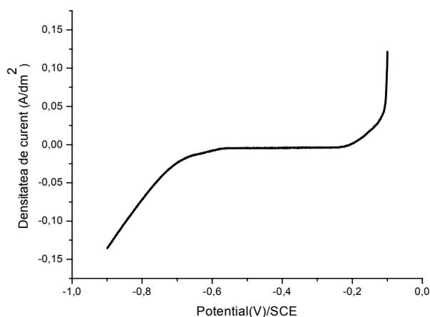
Fig. 1 – Polarization curve for nickel in a Watts bath for the potential range from -100 mV to -1200 mV, 65°C temperature.
