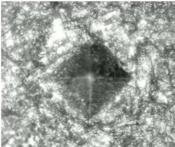
Fig. 4 – Photo of a hardness measurement for a sample of nickel deposited on a copper substrate from a Watts bath with addition of PVP, at -1000 mV potential and 65°C temperature (Shimadzu HMV, 400X optic magnitude).
