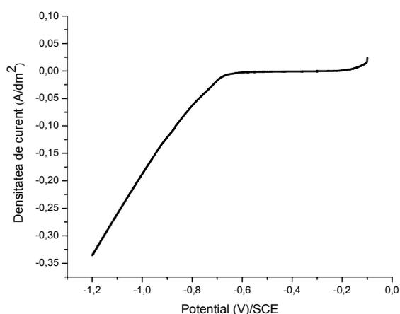
Fig. 2 – Polarization curve for nickel in a Watts bath with 5 gL<sup>-1</sup> PVP adding for the potential range from -100 mV to -1200 mV, 65°C temperature.
