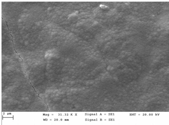
Fig. 6 – SEM image of a nickel layer electrodeposited from a Watts bath with addition of PVP (sample 4) at -1000 mV potential, 65°C temperature, 10 minutes, with magnetic shaking of the electrolyte (SEM-Zeiss EVO 20, 31320X magnification).
