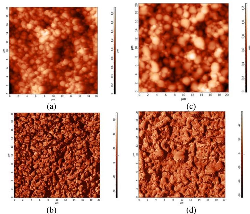
Fig. 5 – AFM topographic and phase images of  $\text{PAT}_1/\text{MMT}$  (a,b) and  $\text{PAT}_2/\text{MMT}$  (c,d) nanocomposites.
