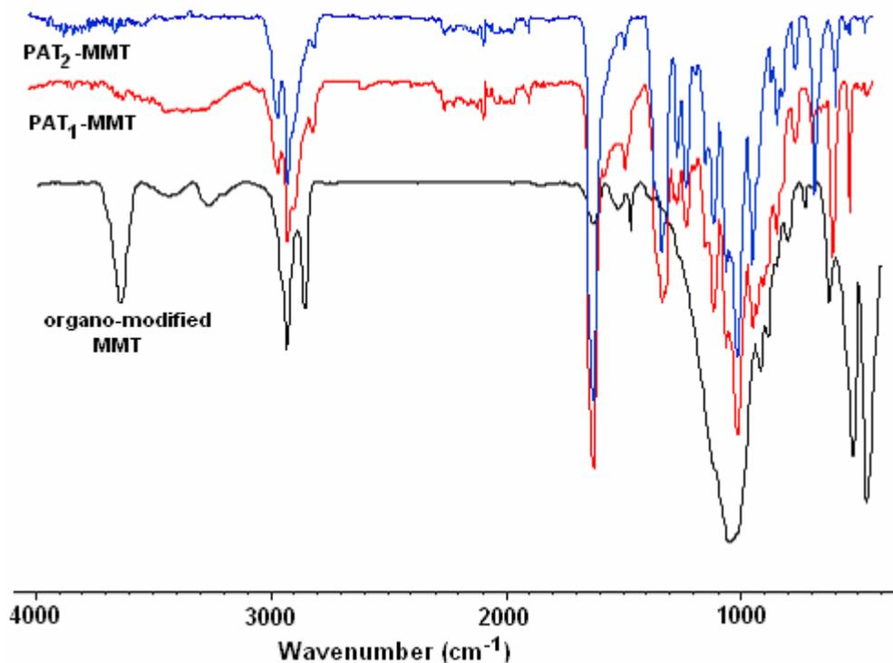
Fig. 4 – FT-IR spectra of organo-modified MMT and triazene polyacrylates/MMT composites.
