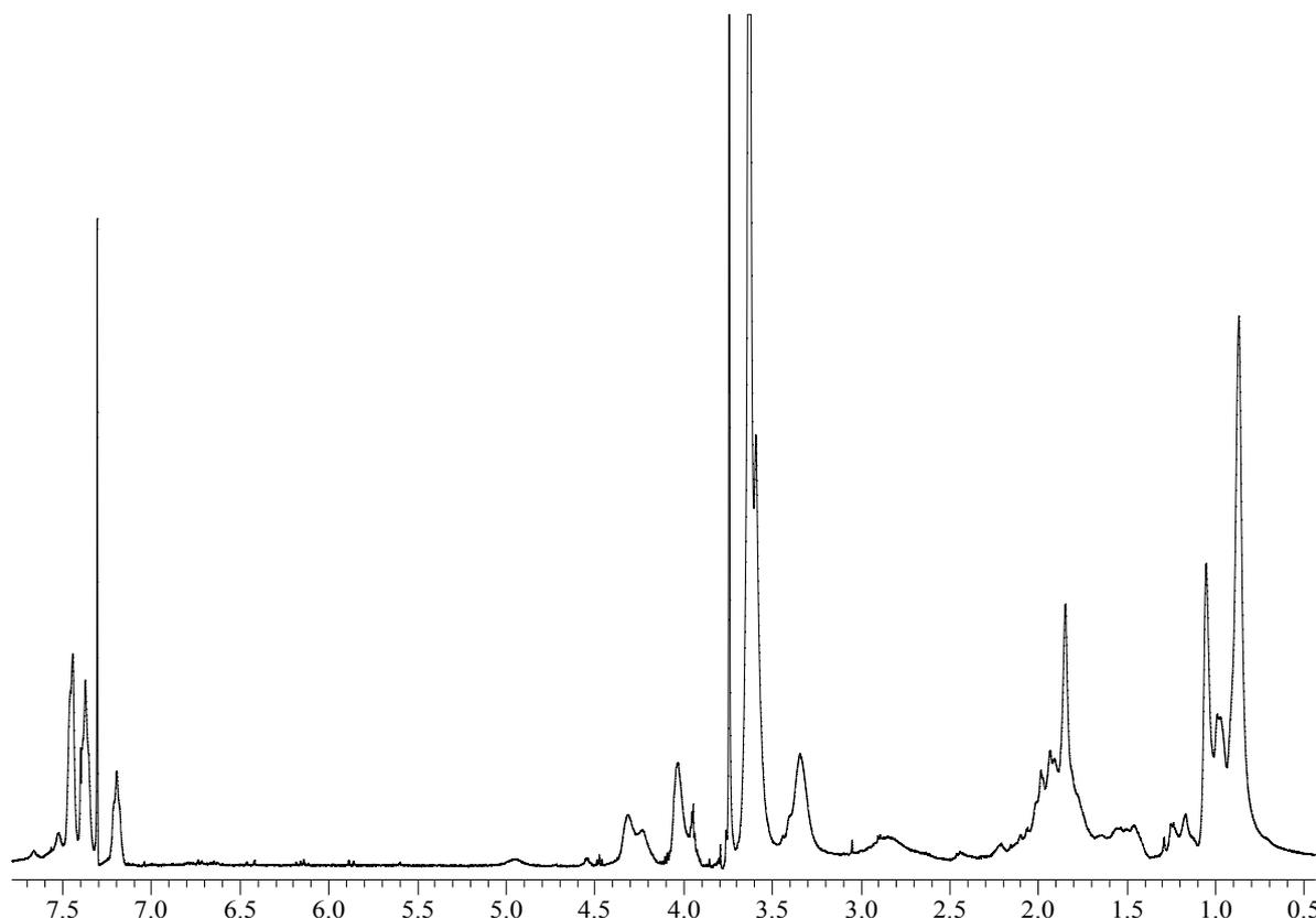
Fig. 1 – <sup>1</sup>H-NMR spectrum of 1-(phenyl)-3-(2 acryloyloxyethyl)-3-methyl triazene-1-co-methyl methacrylate (PAT<sub>1</sub>) in CDCl<sub>3</sub>.
