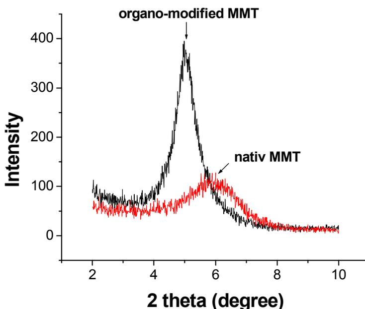
Fig. 2 – XRD patterns of native MMT and organo-modified MMT.
