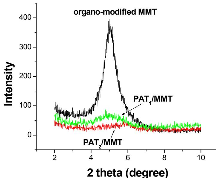
Fig. 3 – X-ray diffraction of modified MMT and the corresponding nanocomposites (PAT<sub>1</sub>/MMT and PAT<sub>2</sub>/MMT).
