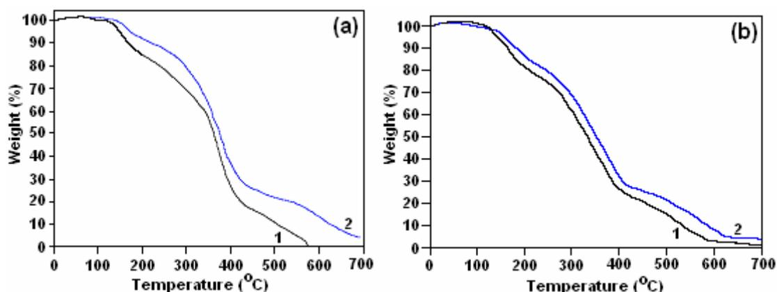
Fig. 7 – TGA curves of (a) PAT<sub>1</sub> (1); PAT<sub>1</sub>/MMT (2); and (b) PAT<sub>2</sub> (1); PAT<sub>2</sub>/MMT (2).
