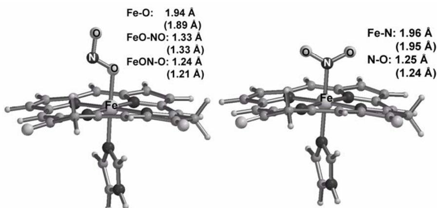
Fig. 3 – Optimized geometries for O- and N-ferrous-nitrite models of the  $cd_1NIR$  active site. Distances for the corresponding ferric-nitrite models are given in parentheses<sup>4</sup>.
