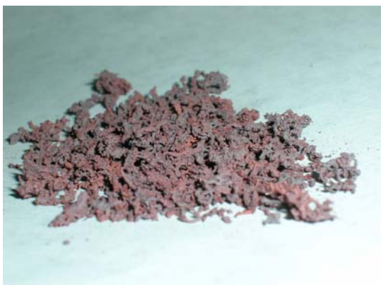
Fig. 2 – Lithium ferrite obtained by the thermal decomposition of the compound [\text{Fe}_{2.5}\text{Li}_{0.5}(\text{CO}(\text{NH}_2)_2)_7](\text{NO}_3)_8 \cdot 6\text{H}_2\text{O} (I) calcinated at 800^\circ\text{C}/1\text{h} .
