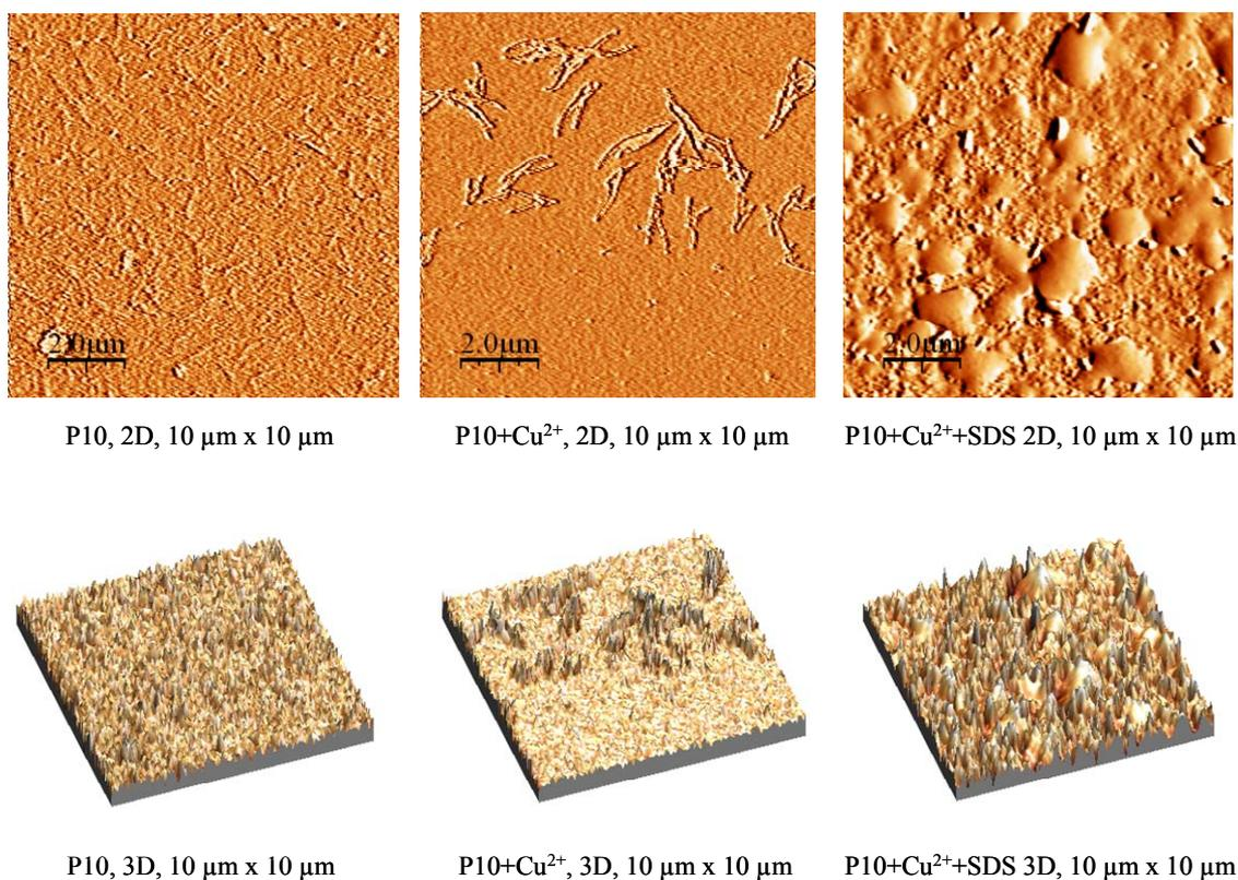
Fig. 4 – Bi- and tridimensional AFM images of pure P10,  $\text{Cu}^{2+}$ -P10 complex in water and in the presence of sodium dodecylsulfate (SDS).
