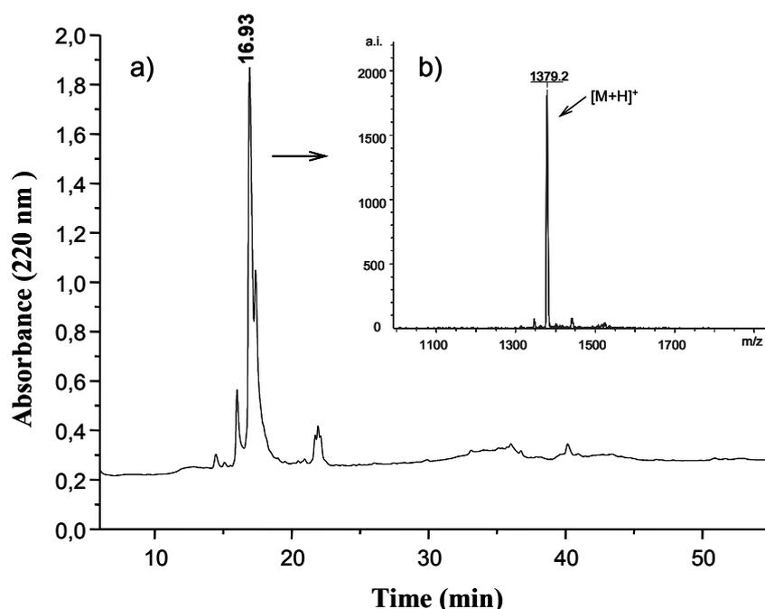
Fig. 1 – RP-HPLC spectrum of the purified P10 (a) as well as its MALDI TOF MS spectrum (b), which show both the molecular weight and the purity of the peptide.
