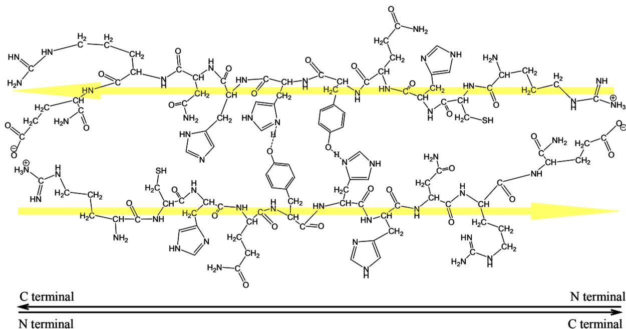
Fig. 3 – The formation of  $\beta$ -sheet conformers of P10 under solid state. The top chain is left side C-terminal; the bottom one is with C-terminal to the right.
