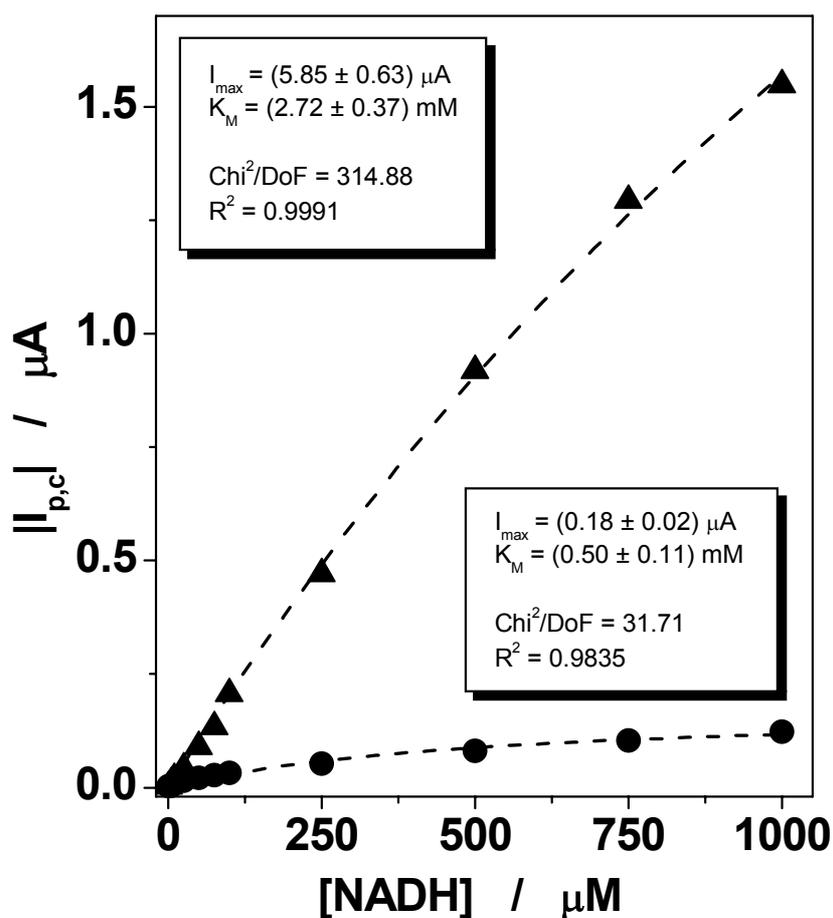
Fig. 4 – Calibration curves for NADH recorded at G/HRP-NADOx (●), and G/RP-HRP-NADOx (▲) electrodes.  $|I_{p,c}|$  stands for the absolute value of the cathodic peak current. *Experimental conditions:* supporting electrolyte, 0.1 M phosphate buffer containing 0.1 M KCl (pH 7.2); applied potential, -50 mV vs. Ag/AgCl, KCl<sub>0.1M</sub>; flow rate, 0.5 ml min<sup>-1</sup>; dispersion coefficient, ~2.
