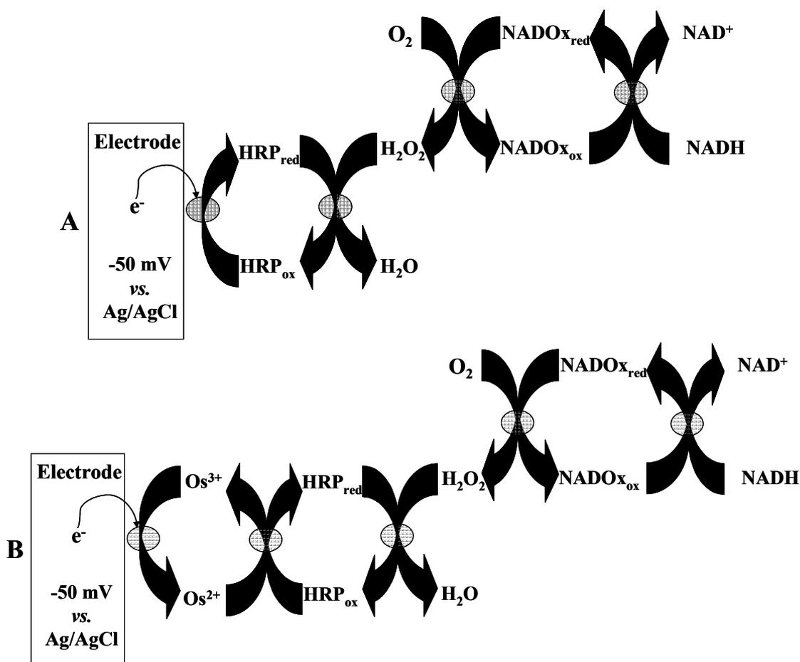
Fig. 1 – The biosensor working principle based on direct (A) and mediated (B) electron transfer.
