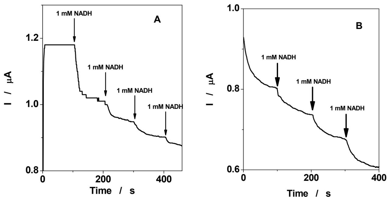
Fig. 3 – Amperometric responses recorded for NADH repetitive additions at G/HRP-NADOx (A) and G/RP-HRP-NADOx (B) electrodes. *Experimental conditions:* supporting electrolyte, 0.1 M phosphate buffer containing 0.1 M KCl (pH 7.2); applied potential, -50 mV vs. Ag/AgCl, KCl<sub>0.1M</sub>.
