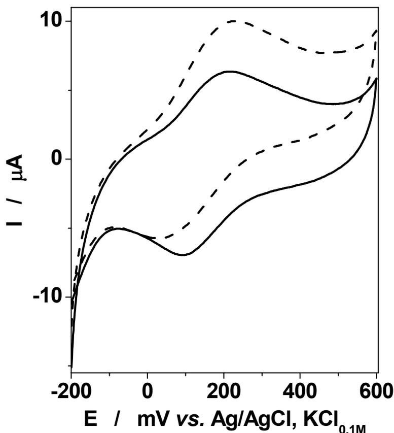
Fig. 2 – Cyclic voltammograms recorded at G/RP-HRP-NAD<sub>ox</sub> electrode in absence (—) and in presence (-----) of NADH. *Experimental conditions*: supporting electrolyte, 0.1 M phosphate buffer containing 0.1 M KCl (pH 7.2); starting potential, -200 mV vs. Ag/AgCl, KCl<sub>0.1M</sub>; [NADH], 1 mM; scan rate, 5 mV s<sup>-1</sup>.
