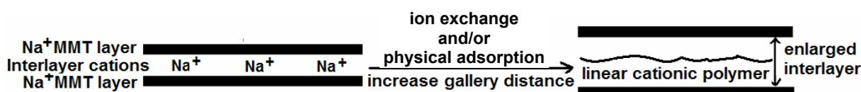
Fig. 3 – Schematic structure of unmodified clay (MMT) and polymer-intercalated MMT.
