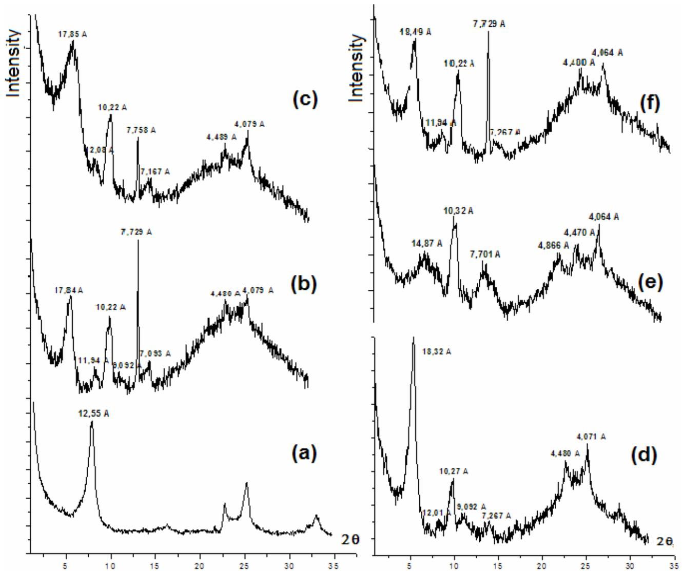
Fig. 2 – The XRD diffractogram of MMT (a); COL/CH/MMT/PL (b); COL/CH/MMT (c); CH/MMT/PL (d); CH/MMT (e); COL/MMT/PL (f).
