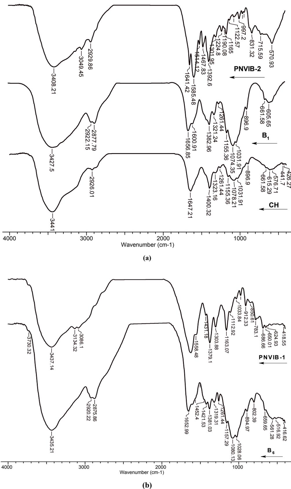
Fig. 2 – FT-IR spectra of: a) chitosan, B<sub>1</sub> complex and PNViB-2; b) B<sub>6</sub> complex and PNViB-1.
