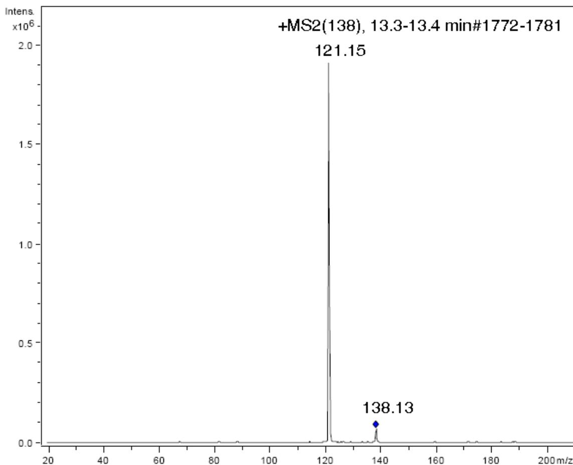
Fig. 3 – Fragmentation of protonated *Tyramine*.
