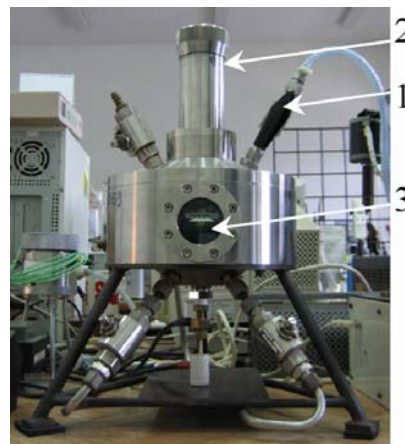
Fig. 1 – Test cell for MESG measurement: 1–admission valve; 2–micrometric screw; 3–observation window.
