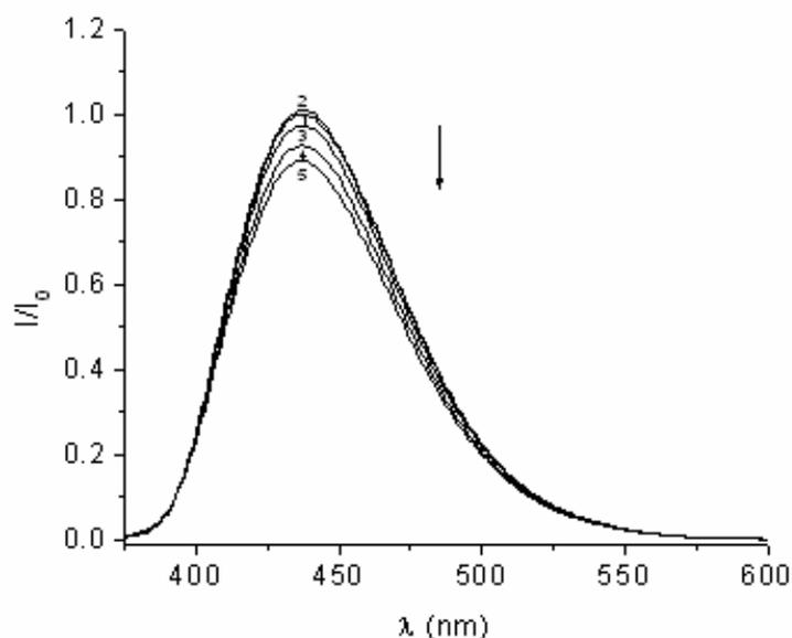
Fig. 4 – Normalized fluorescence spectra of BzCum ( $2.76 \times 10^{-5} \text{ M}$ ) in the presence of different SDS concentrations. [SDS]: (1) 0 M; (2)  $4.06 \times 10^{-3} \text{ M}$ ; (3)  $9.81 \times 10^{-3} \text{ M}$ ; (4)  $1.95 \times 10^{-2} \text{ M}$ ; (5)  $2.92 \times 10^{-2} \text{ M}$ ;  $\lambda_{\text{ex}} = 360 \text{ nm}$ .
