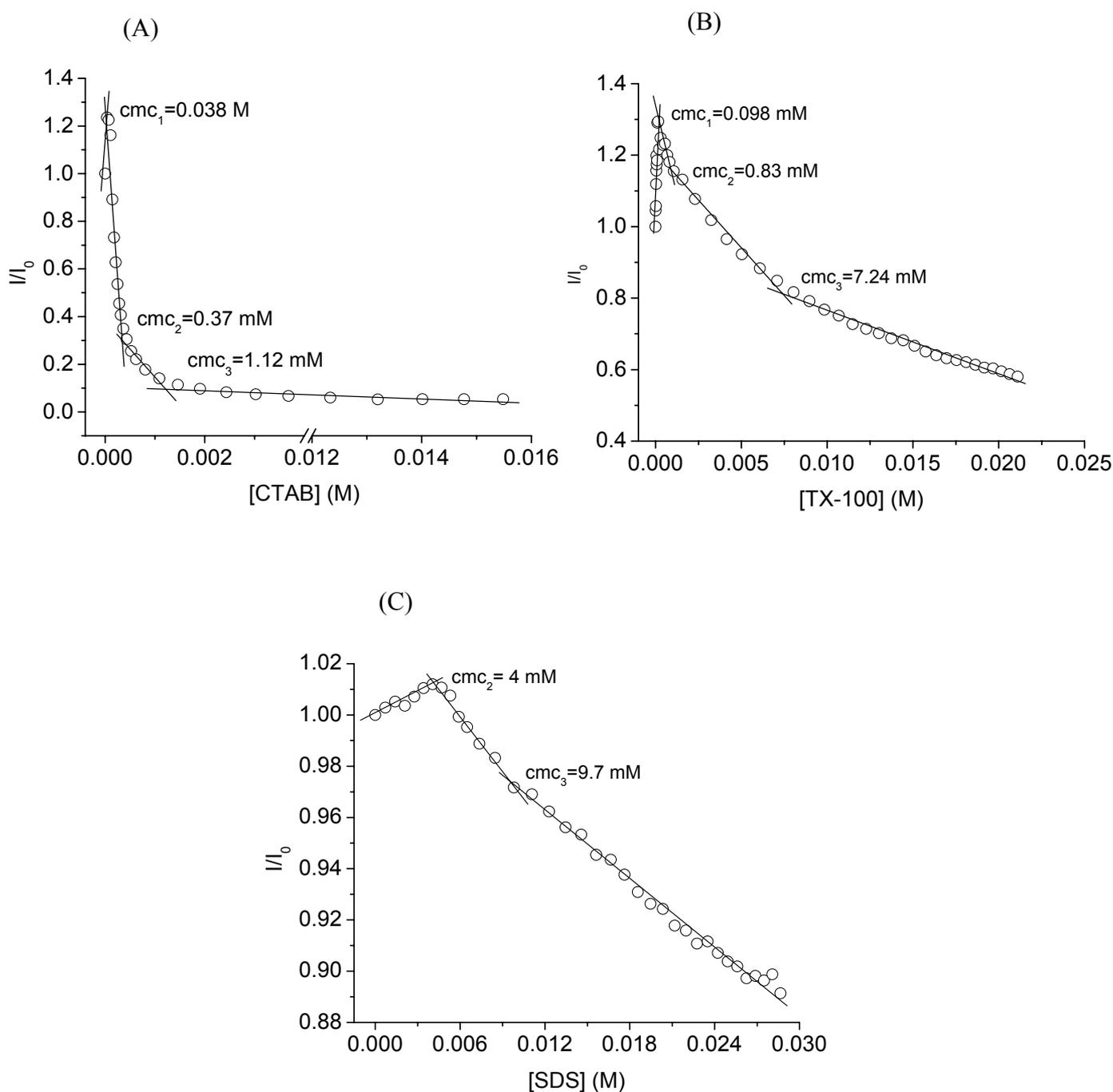
Fig. 5 – Variation of normalized fluorescence of BzCum as a function of CTAB (A), TX-100 (B) and SDS (C) concentrations.
