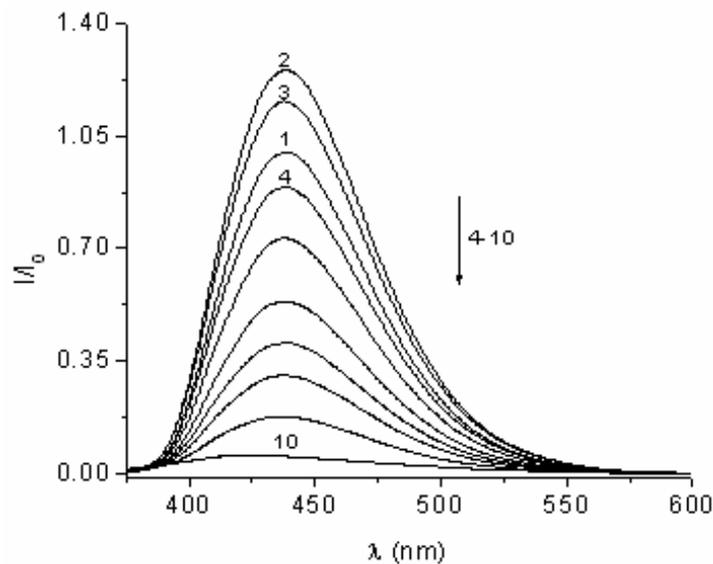
Fig. 2 – Normalized fluorescence spectra of BzCum ( $2.76 \times 10^{-5}$  M) in the presence of different CTAB concentrations. [CTAB]: (1) 0 M; (2)  $3.65 \times 10^{-5}$  M; (3)  $7.25 \times 10^{-5}$  M; (4)  $1.43 \times 10^{-4}$  M; (5)  $1.78 \times 10^{-4}$  M; (6)  $2.46 \times 10^{-4}$  M; (7)  $3.14 \times 10^{-4}$  M; (8)  $4.28 \times 10^{-4}$  M; (9)  $8.08 \times 10^{-4}$  M; (10)  $1.47 \times 10^{-2}$  M.  $\lambda_{\text{ex}} = 360$  nm.
