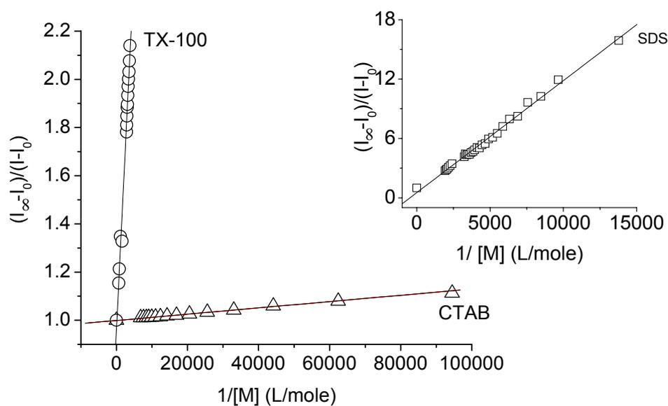
Fig. 7 – Plot of  $(I_\infty - I_0)/(I - I_0)$  versus  $1/[M]$  for BzCum in CTAB ( $\Delta$ ), Triton-X ( $\circ$ ) and SDS ( $\square$ ) at pH=10. The lines corresponds to the linear fits using eq. (5).
