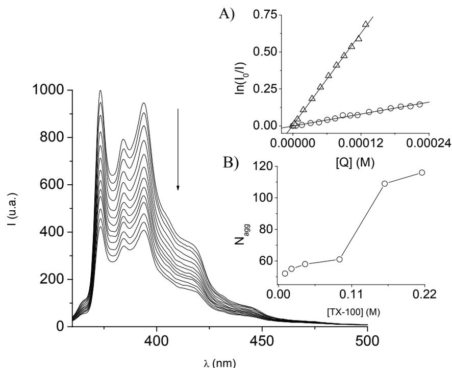
Fig. 6 – Fluorescence quenching of pyrene in TX-100 10 mM by various concentrations of benzophenone. Inset (A) plot of the  $\ln(I_0/I)$  for pyrene in the presence of different benzophenone concentrations in 10 mM ( $\Delta$ ) and 92 mM ( $\circ$ ) Tx-100. The solid lines represent the fits using Eq. (3). Inset (B) the dependence of the aggregation numbers of TX-100 with the surfactant concentration in buffered solutions.
