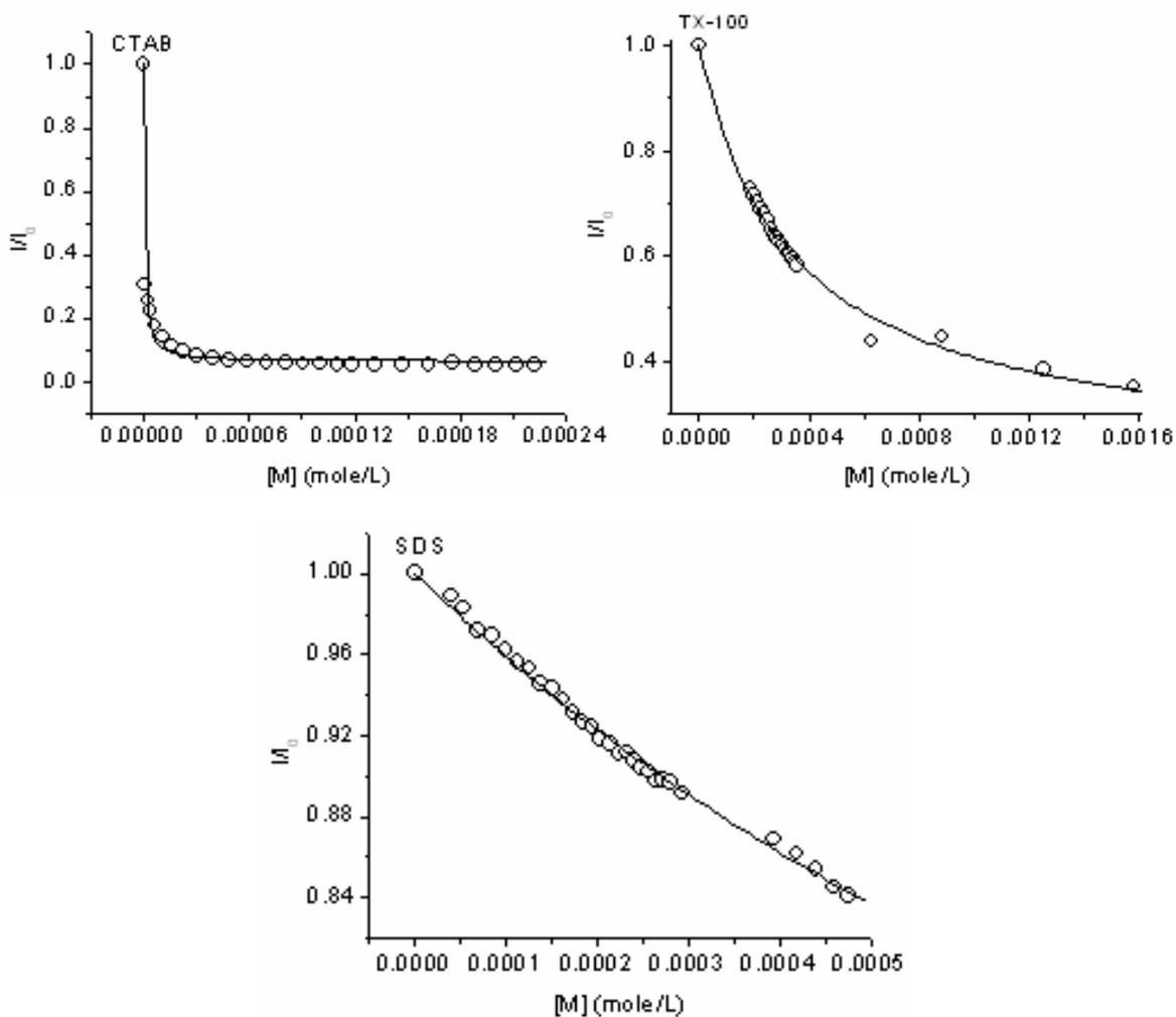
Fig. 8 – Best fit of the plot of the normalized intensity versus micelle concentration using eq. (4).
