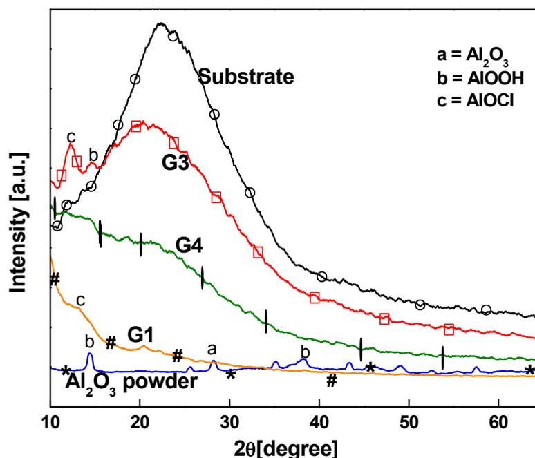
Fig. 1 – XRD patterns of alumina films deposited on microglass substrates by SPD.
