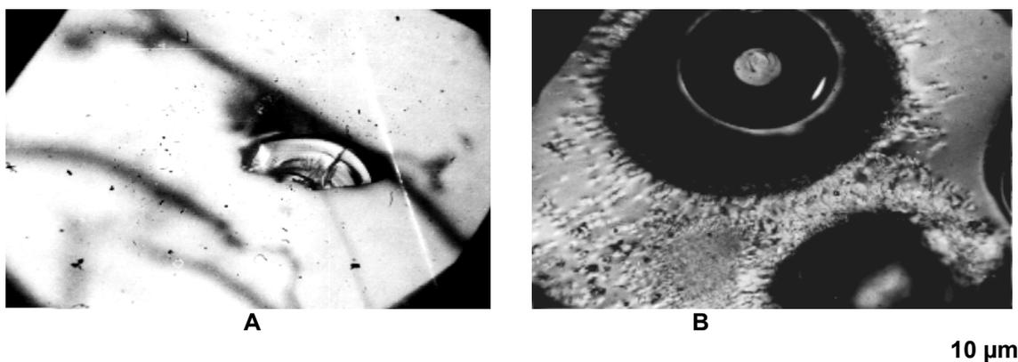
Fig. 5 – Photomicrographs of some vitreous carbon nanocomposites, polarized light, oil immersion, nichols, 250x. (A). Isotropic matrix of vitreous carbon with pyrocarbon buds having different degrees of structural orientation (B). Needle textures of vitreous graphitized carbon samples with different size and anisotropic intensity.<sup>16</sup>
