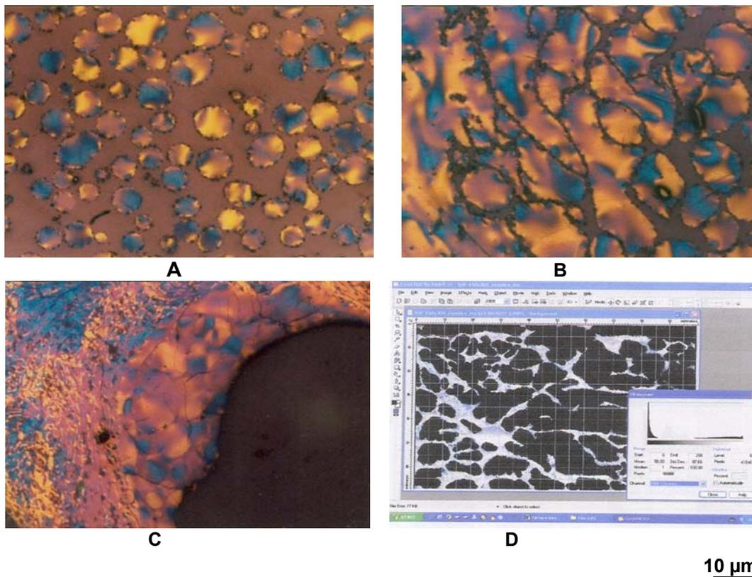
Fig. 4 – Photomicrographs of some carbon-carbon nanocomposites, polarized light, oil immersion, nichols, 250x. (A). Dispersed mesophase pitch units (B). Mesophase pitch coalescence in larger units (C). Microstructure aspect of anisotropic coke formation (D). Statistically evaluation of mesophase units on size distribution.<sup>15</sup>
