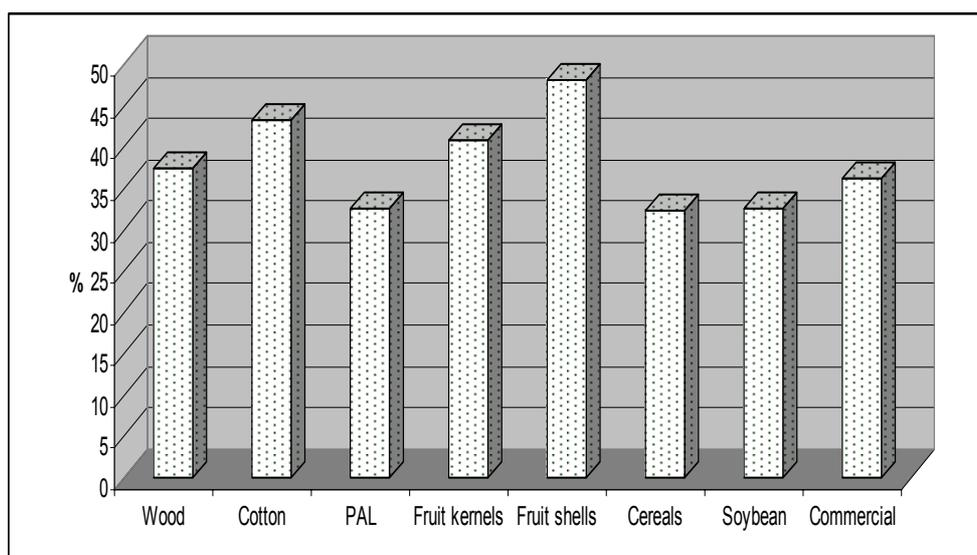
Fig. 1 – Activated carbon inter-grain porosity < 2.5  $\mu\text{m}$  distribution.
