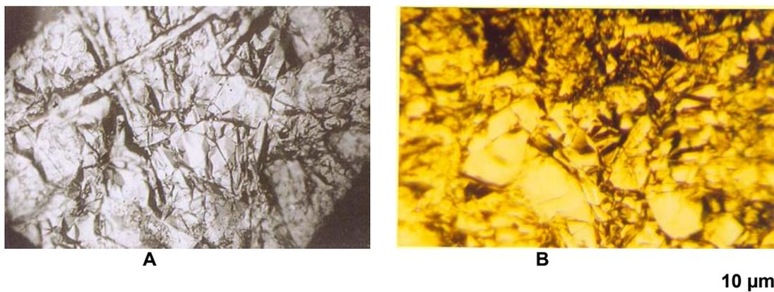
Fig. 3 – Photomicrographs of some graphite intercalated compounds, polarized light, oil immersion, nichols, 250x. (A). Smaller units less orientated and partially banded. (B). Better organization in expanded intercalated units, packed in sheets without network defects.<sup>14</sup>
