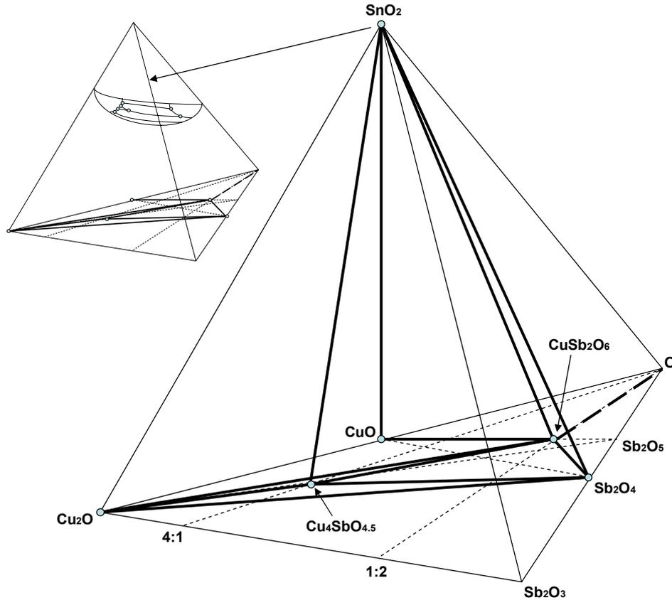
Fig. 1 – The  $T$ - $x$ - $y$ - $z$  diagram of ternary SnO<sub>2</sub> – Sb<sub>2</sub>O<sub>3</sub> – Cu<sub>2</sub>O – O system.
