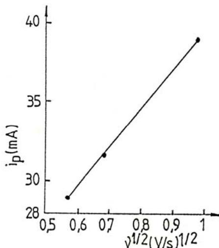
Fig. 3 – Dependence of the anodic peak current ( $i_{pa}$ ) on square root of the scan rate ( $v^{1/2}$ ) for the cyclic voltammograms recorded in a cryolite-alumina melt at 980<sup>0</sup>C with S2-anode.
