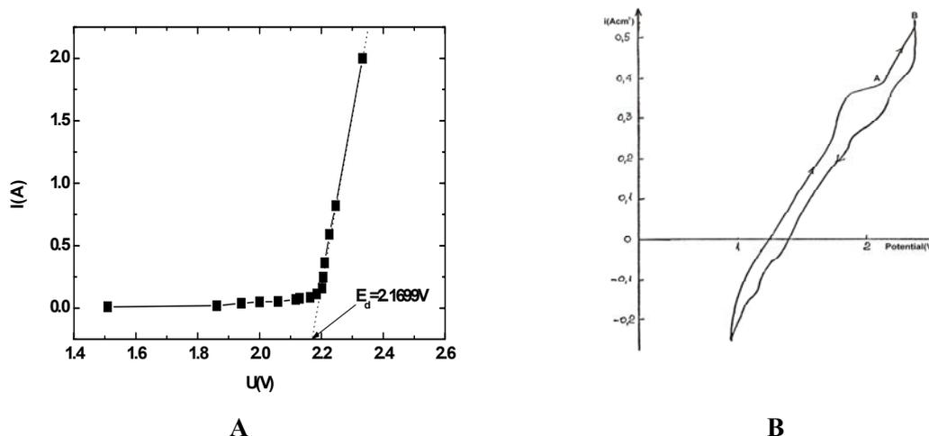
Fig. 2 – Electrochemical data obtained on S2-anode in Na<sub>3</sub>AlF<sub>6</sub>-CaF<sub>2</sub>-Al<sub>2</sub>O<sub>3</sub> melt at 980<sup>0</sup>C and 0.8Acm<sup>-2</sup>:
