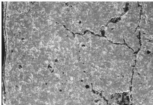
Fig. 6 – The SEM micrograph image of the active surface of S2 inert anode after electrolysis.
