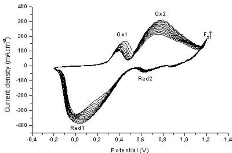
Fig. 7 – The cyclic voltammogram obtained for the solubility of S2 inert anode in cryolite-alumina melt at 980°C; QRE=Pt wire ( $\phi=2\text{mm}$ ), CE=GC wire ( $\phi=2\text{mm}$ );  $v=50\text{-}200\text{mVs}^{-1}$ .
