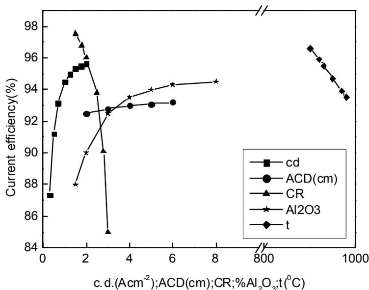
Fig. 4 – Evolution of the current efficiency of S2 with current density (cd), anode-cathode distance (ACD), cryolite ratio ( $\text{CR} = \text{molNaF/molAlF}_3$ ), concentration of  $\text{Al}_2\text{O}_3$  in the electrolyte bath and the temperature (t).
