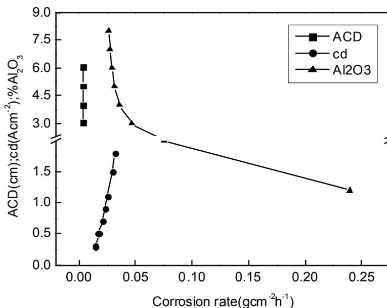
Fig. 5 – Corrosion rate of S2 as a function of the current density (cd), anode-cathode distance (ACD) and wt% Al<sub>2</sub>O<sub>3</sub>.
