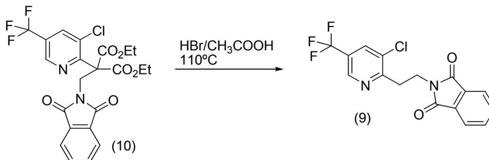
Scheme 5. Synthesis of 2-(2-(3-chloro-5-(trifluoromethyl)pyridin-2-yl)ethyl)isoindoline-1,3-dione
