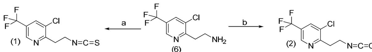
a: X=S, CSCI<sub>2</sub>, DCM/NaHCO<sub>3</sub>, 0°C; b: X=O, OC(OCCl<sub>3</sub>)<sub>2</sub>, DCM/NaHCO<sub>3</sub>, 0°C
