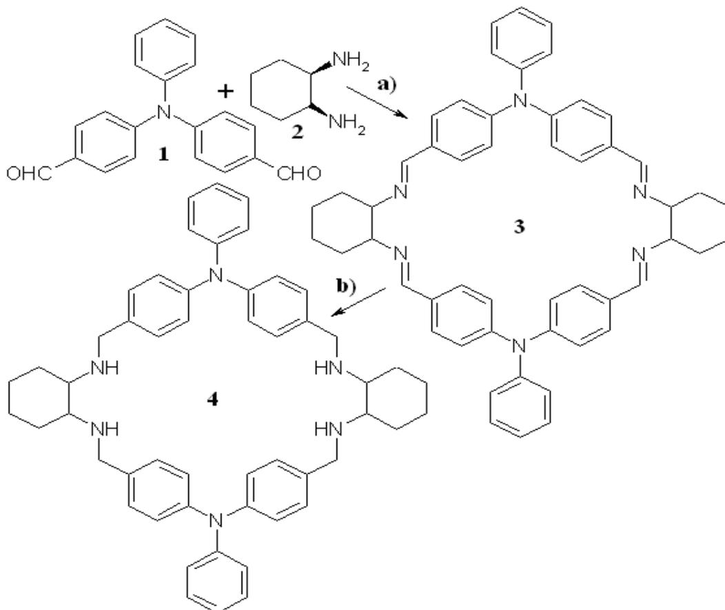
Scheme 1 – Synthesis of triphenylamine-based rhombimine and rhombamine macrocycles:
