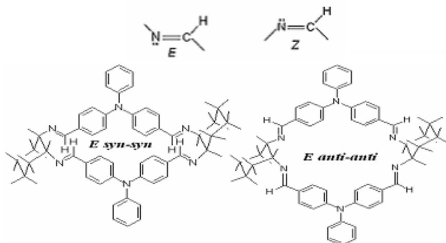
Fig. 5 – *E/Z* configuration and *syn/anti* conformation isomers.
