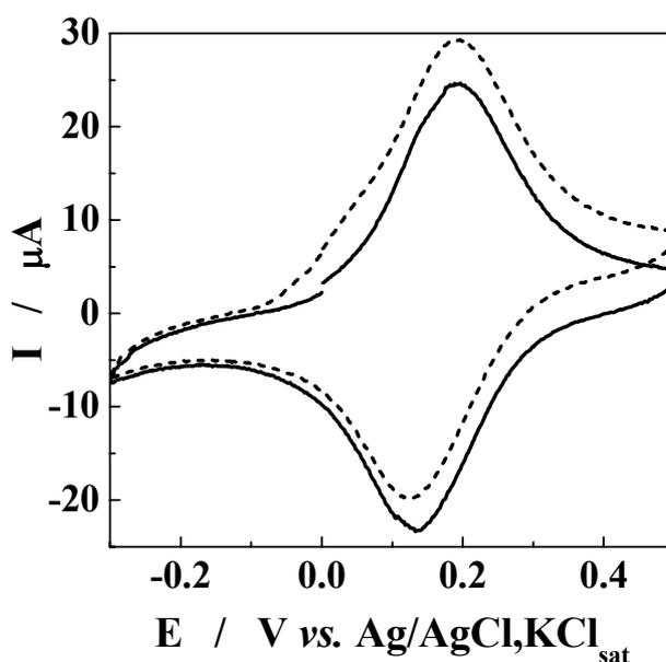
Fig. 4 – Cyclic voltammograms recorded at G/Os-HRP bioelectrode in PB solution (—) and in PB solution containing 1 mM AA (----). Experimental conditions: potential scan rate, 5 mV/s; starting potential,  $-0.300$  V vs. Ag/AgCl/KCl<sub>sat</sub>.
