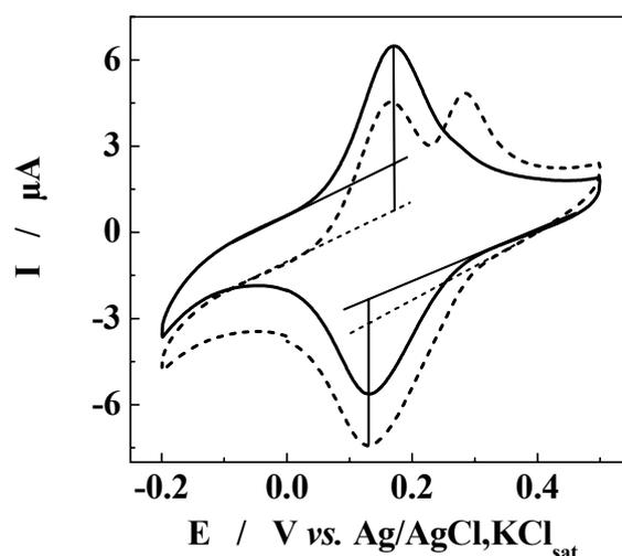
Fig. 3 – Cyclic voltammograms recorded at G/Os-HRP bioelectrode in PB solution (—) and in PB solution containing 0.1 XOD U/mL and 0.41 mM XA (----). Experimental conditions: potential scan rate, 0.005 V/s; starting potential, -0.2 V vs. Ag/AgCl/KCl<sub>sat</sub>.
