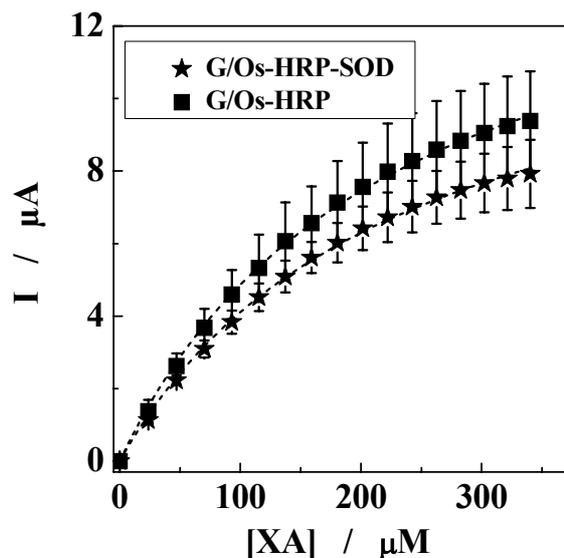
Fig. 1 – Calibration curves for G/Os-HRP and G/Os-HRP-SOD biosensors. Experimental conditions: applied potential,  $-0.100\text{ V vs. Ag/AgCl, KCl}_{\text{sat}}$ ; supporting electrolyte,  $0.1\text{ M PB}$  containing  $0.1\text{ XOD U/mL}$  ( $\text{pH } 7.5$ ); stirring rate,  $1500\text{ rpm}$ .
