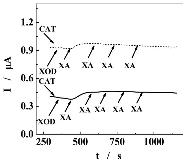
Fig. 2 – Amperometric responses recorded for G/Os-HRP-SOD (-----) and G/Os-HRP (—) biosensors for successive additions of  $23\text{ }\mu\text{M XA}$  in PB solution ( $\text{pH } 7.5$ ) containing CAT ( $295\text{ U/mL}$ ) and XOD ( $0.1\text{ U/mL}$ ). Experimental conditions: same as in Fig. 1.
