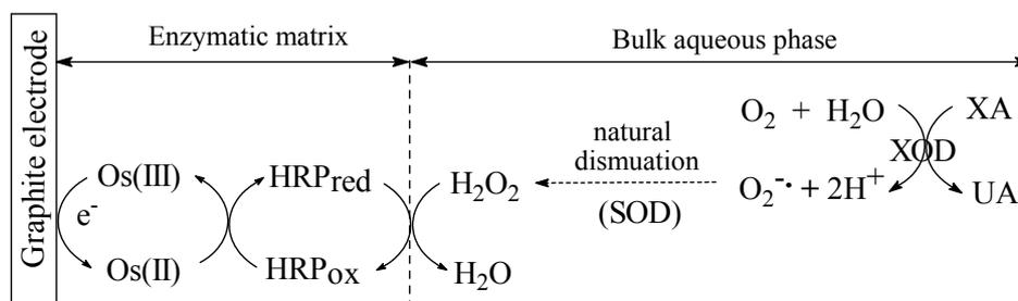
Fig. 5 – Detection scheme of  $H_2O_2$ , generated by the XA-XOD enzymatic system.
