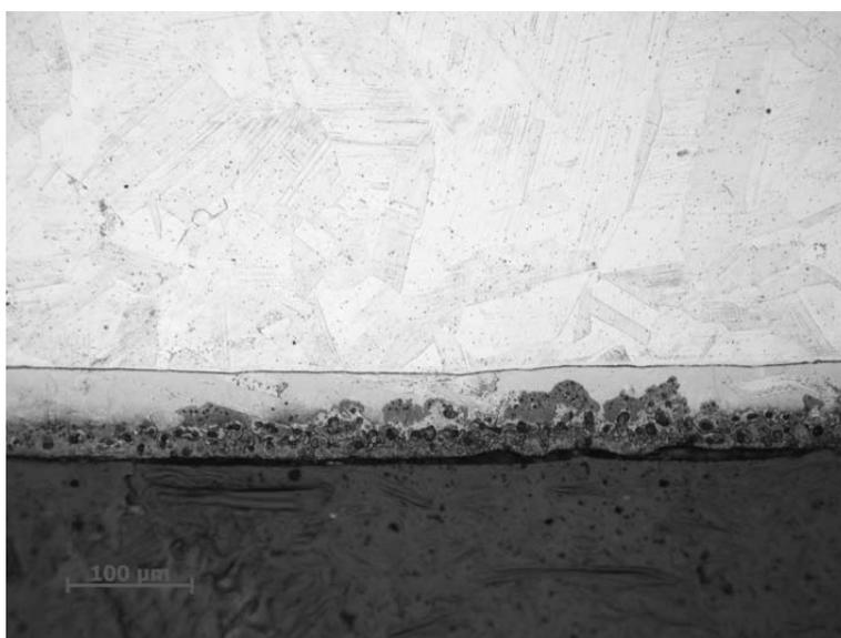
Fig. 1 – OM cross-sectional views of the plasma nitrided austenitic stainless steel.
