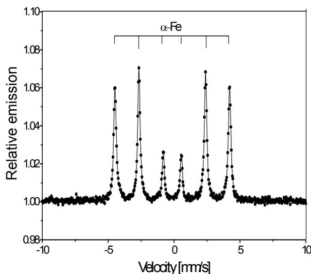
Fig. 7 – CEMS spectrum of a corroded sample in a solution with  $10^{-3}$   $\text{HN}_3$  concentration with NCBSA inhibitor (● data; — fit; ---  $\alpha$ -Fe).
