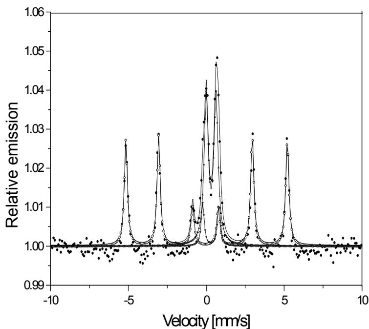
Fig. 9 – CEMS spectrum of a corroded sample in a 1M HCl solution with APM inhibitor (• data; — fit; -o-  $\alpha$ -Fe; - $\Delta$ - doublet 1; - $\nabla$ - doublet 2).
