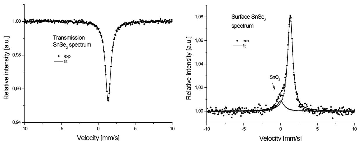
Fig. 10 – Spectra of SnSe<sub>2</sub> bulk sample obtained by TMS (left) and CEMS (right).
