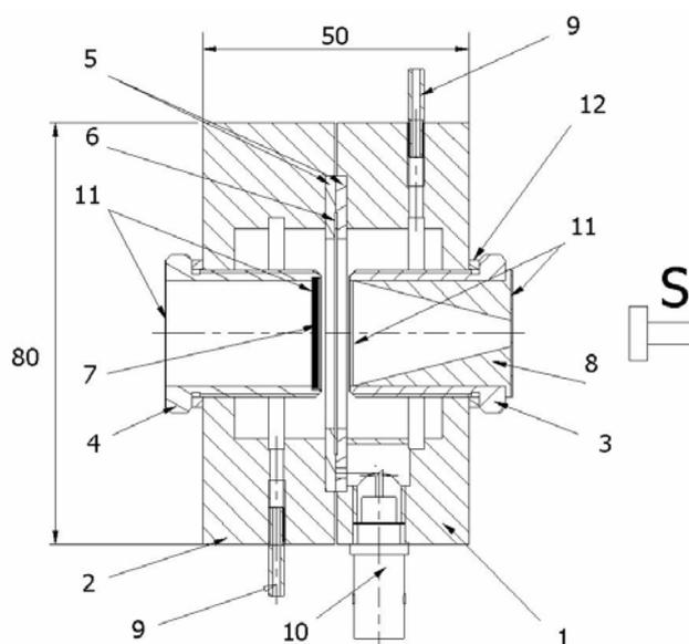
Fig. 3 – The cross section of the versatile flow-gas proportional counter, 1 and 2 main parts of the counter, 3 input piece, 4 sample holder, 5 teflon insulator, 6 anodic ring, 7 sample, 8 collimator, 9 gas connection, 10 high voltage connector, 11 mylar windows, 12 tightness piece, S Mössbauer source.
