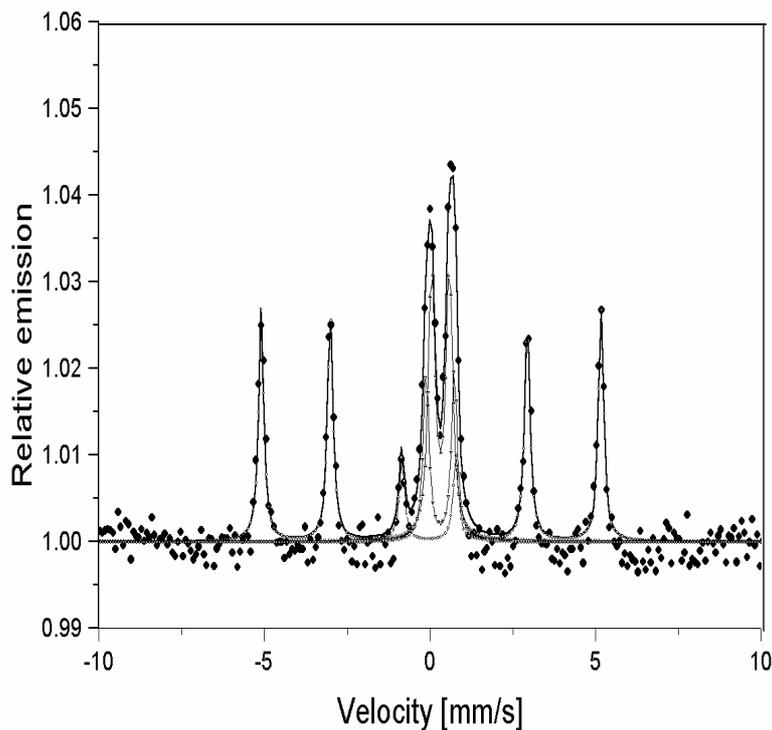
Fig. 8 – CEMS spectrum of a corroded sample in a 1 M HCl solution (• data; — fit; -o-  $\alpha$ -Fe; - $\Delta$ - doublet 1; - $\nabla$ - doublet 2).
