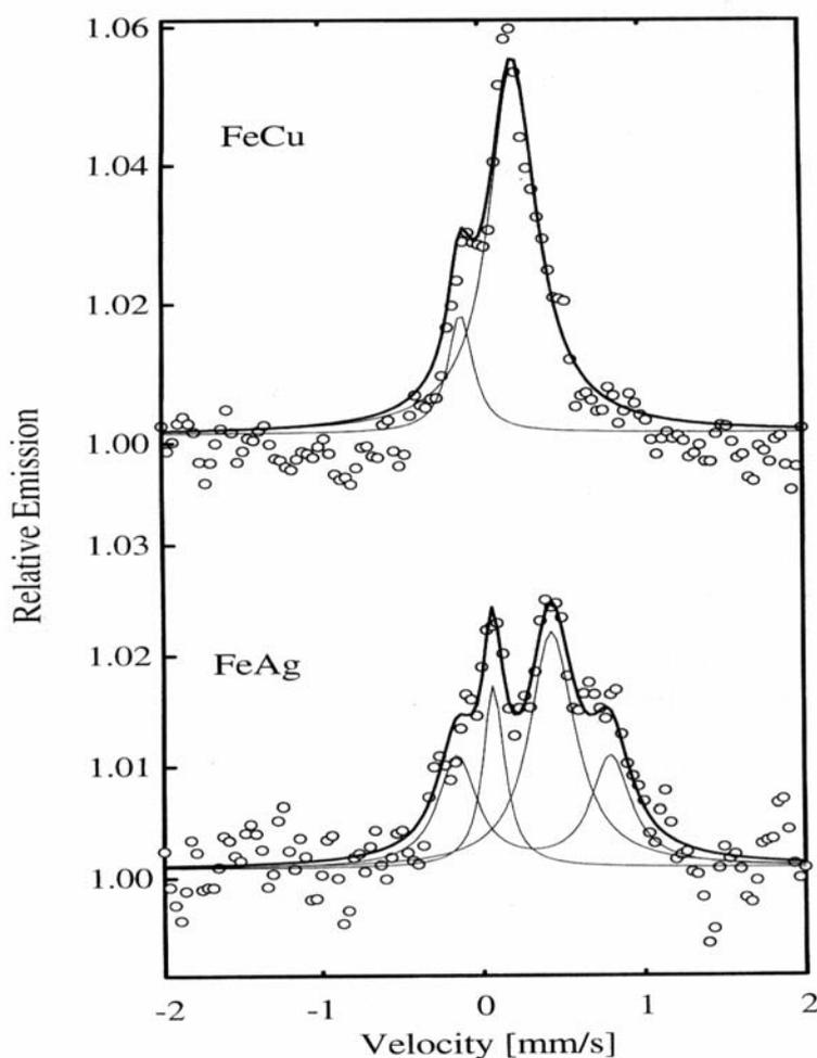
Fig. 5 – CEMS spectra of diluted granular films of Cu-Fe and Ag-Fe (iron content  $\leq 2\%$ ) produced using  $^{57}\text{Fe}$  implantation Cu (Ag) films, previously grown by laser ablation.
