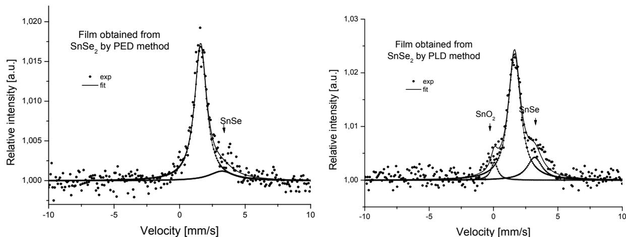
Fig. 11 – CEMS spectra of the films deposited from SnSe<sub>2</sub> by PED and PLD methods.
