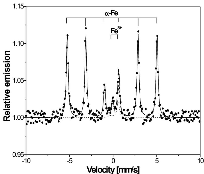
Fig. 6 – CEMS spectrum of a Fe-C steel sample corroded in a solution with  $10^{-3}$   $\text{NH}_3$  concentration (• data; — fit; ---  $\text{Fe}^{3+}$ ; ···  $\alpha\text{-Fe}$ ).
