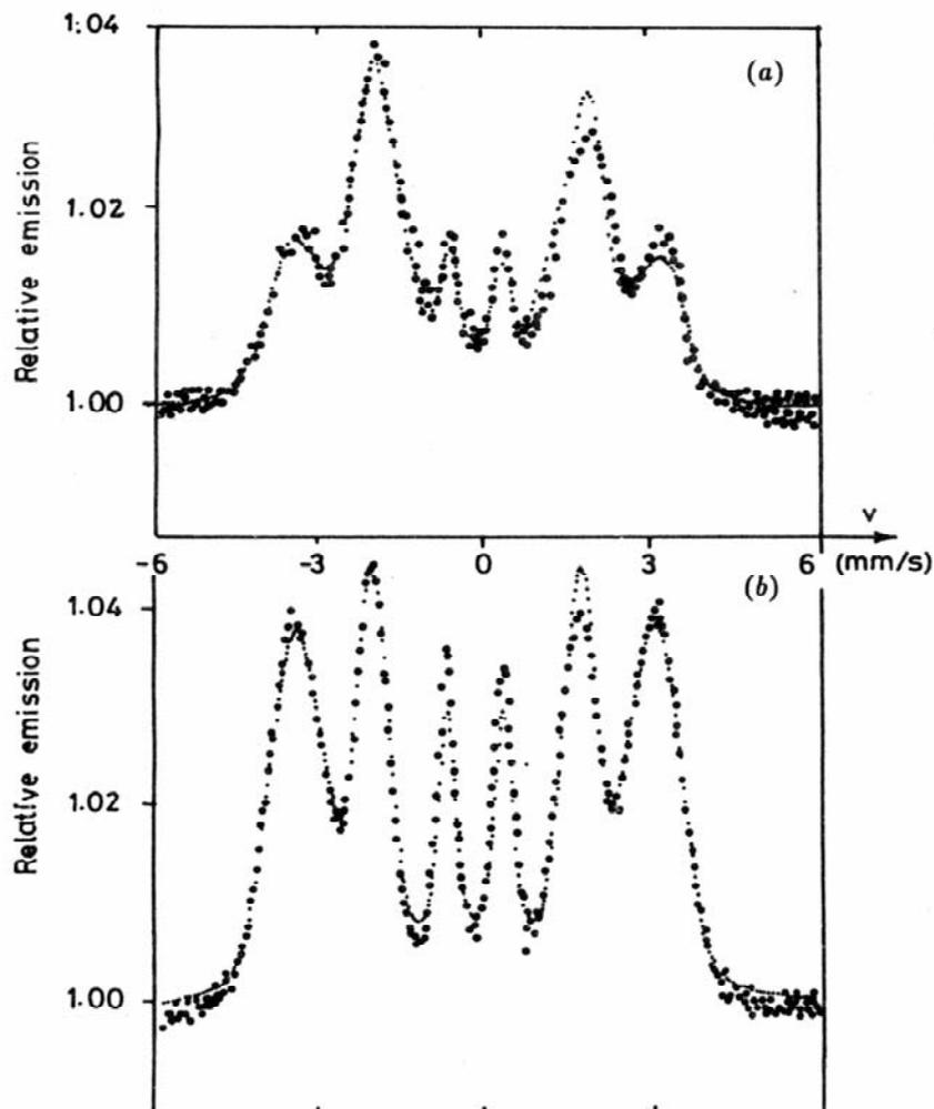
Fig. 4 – Room temperature CEMS spectra for both the (a) film and (b) the ribbon target of Metglass 2605 SC ( $\text{Fe}_{81}\text{B}_{13.5}\text{Si}_{3.5}\text{C}_2$ ).
