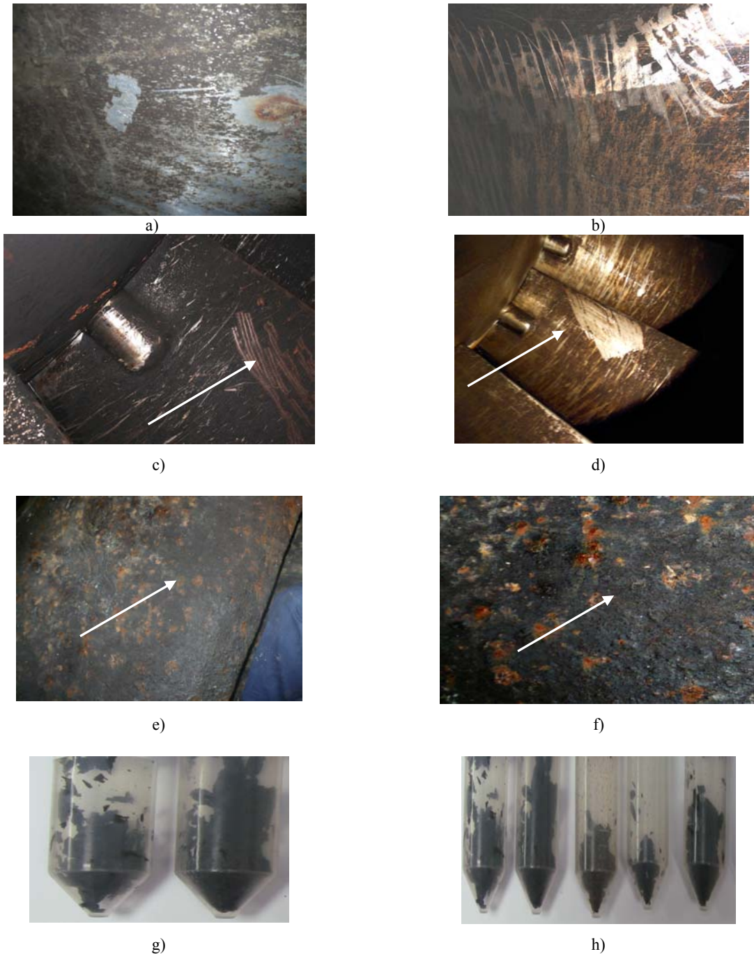
Fig. 2 – Photographs of biofilms (microbe slimes) grown on metallic surfaces: a) biofilm grown on surface of paddle wheel; b) biofilm grown on surface of paddle wheel; c) biofilm grown on aggregates (white arrow – collecting point); d) biofilm grown on tapered aggregate (site III) (white arrow – collecting point); e) corroded zones of hydro-aggregates; f) damages of as a result of corrosion (white arrow – “tubercles”); g) biofilm and pit scraped from collecting point of aggregates; h) biofilm and pit scraped from collecting point of aggregates.
