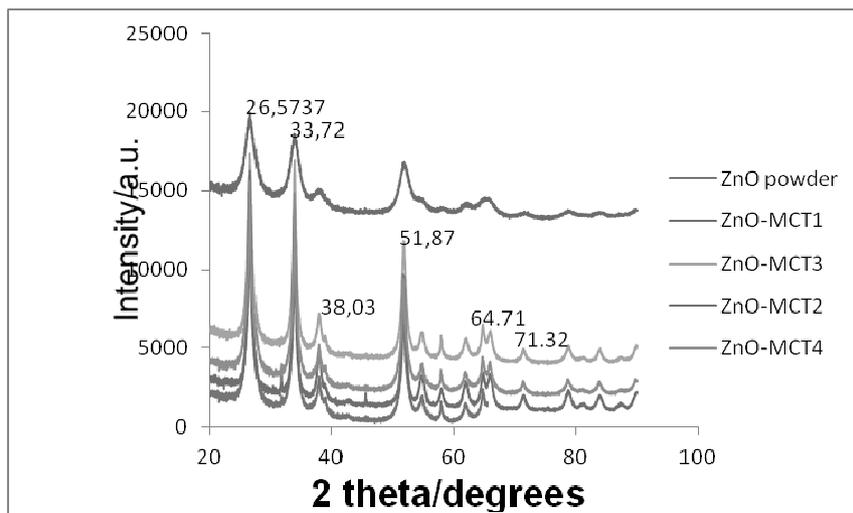
Fig. 6 – XRD pattern of nano ZnO entrapped in different concentrations of MCT; a – ZnO-MCT<sub>1</sub>; b – ZnO-MCT<sub>2</sub>; c – ZnO-MCT<sub>3</sub>; d – ZnO-MCT<sub>4</sub>.
