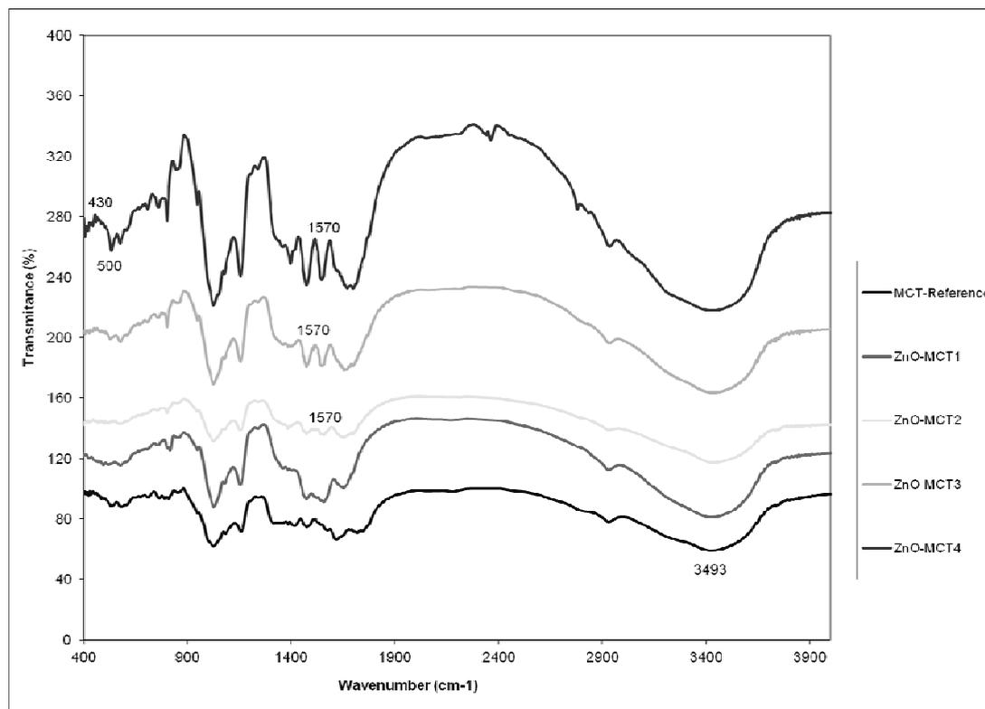
Fig. 7 – FT-IR Spectra of ZnO powders (ZnO-MCT1; ZnO-MCT2, ZnO-MCT3; ZnO-MCT4), compared with MCT spectrum.
