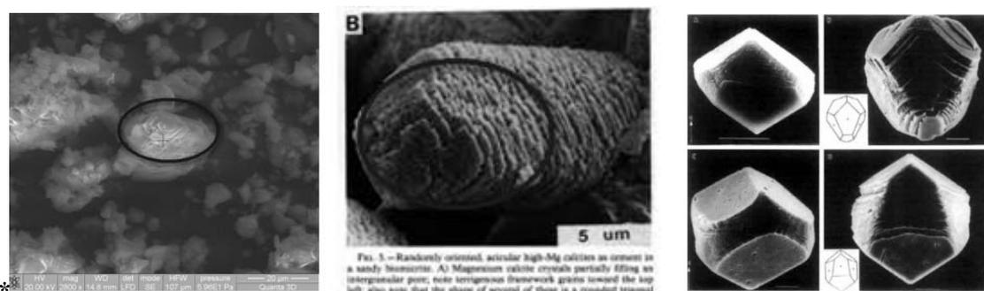
Fig. 1 – Similarities between studied lamellar structures of ZnO nanoparticles entrapped in MCT matrix and calcites from the literature.<sup>26</sup>
