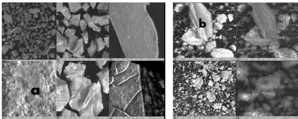
Fig. 2 – Scanning electron micrograph of zinc oxide embodied in: **a.**  $\text{MCT}_1$  and **b.**  $\text{MCT}_2$  matrices.
