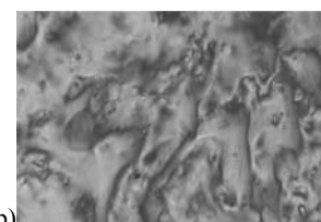
Fig. 4 – Optical micrograph of 4 : a) – smectic A phase at 155.5 °C; b) – nematic phase ( marbled texture) at 166.2 °C.
