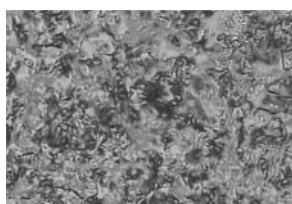
Fig. 2 – Optical texture (schlieren) of a nematic phase of 17 at 132.8 °C.
