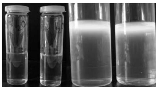
Fig. 4 – 3T1 and 3T2 in water in the day light (left side) and under excitation with a 365 nm UV lamp (right side).
