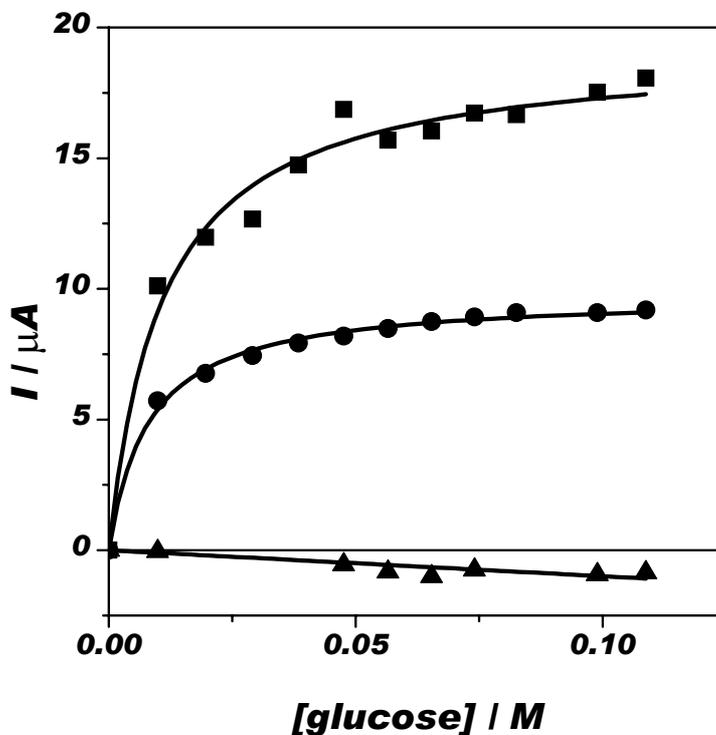
Fig. 3 – Amperometric calibration plot for glucose at Cu/CuO/Gox electrode. Experimental conditions: supporting electrolyte, phosphate buffer 0.1 M (pH 7); applied potential, -0.1 ( $\blacktriangle$ ), 0 V ( $\bullet$ ) and +0.1 V ( $\blacksquare$ ) vs. Ag/AgCl,  $\text{KCl}_{\text{sat}}$ ; continuous stirred aerated solution.
