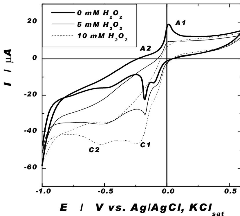
Fig. 2 – The electrocatalytic effect of Cu/CuO modified electrode towards  $\text{H}_2\text{O}_2$  electroreduction. Experimental conditions: electrolyte, phosphate buffer 0.1 M (pH 7); starting potential, -1 V vs. Ag/AgCl,  $\text{KCl}_{\text{sat}}$ ; scan rate,  $5 \text{ mV s}^{-1}$ .
