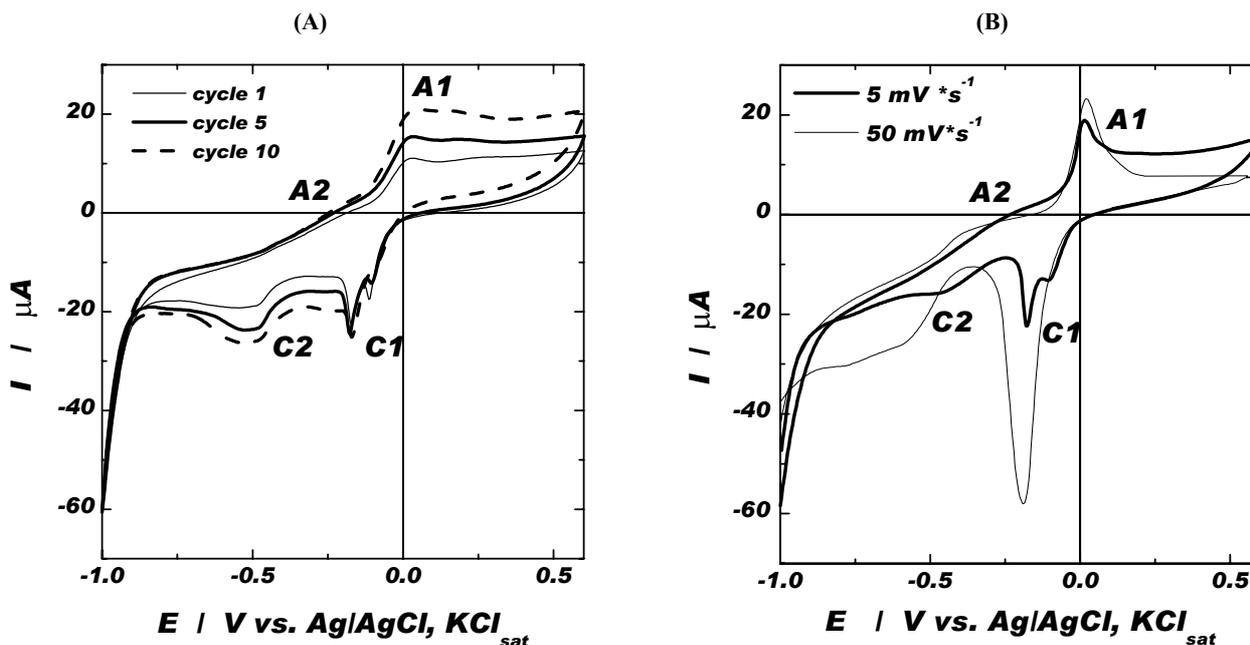
Fig. 1 – (A) Preparation of Cu/CuO modified electrode and (B) the influence of the scan rate on the preparation of the Cu/CuO modified electrode. Experimental conditions: electrolyte, phosphate buffer 0.1 M (pH 7); starting potential, -1 V vs. Ag/AgCl, KCl<sub>sat</sub>; scan rate, 5 mV s<sup>-1</sup> (A, B), 50 mV s<sup>-1</sup> (B, thin line); number of cycles, 1, 5, 10 (A), 20 (B).
