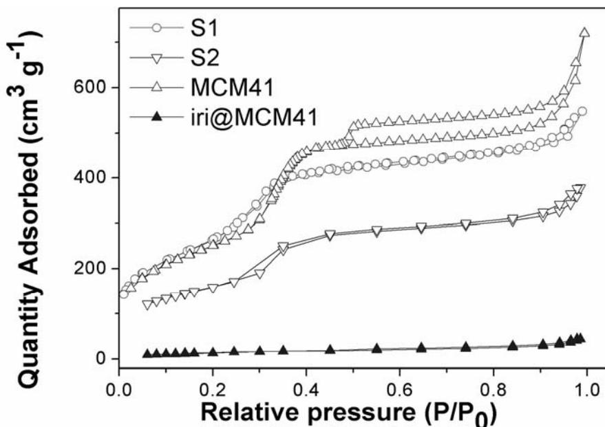
Fig. 2 – N<sub>2</sub> adsorption/desorption isotherms of MCM-41-type supports and iri@MCM-41 hybrid sample.
