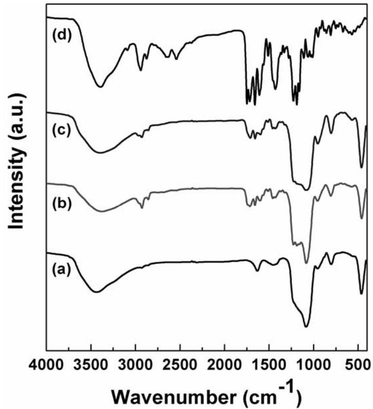
Fig. 3 – FTIR spectra of S1 support (a), iri@S1 hybrid (b), iri@S1f, the hybrid isolated after the delivery experiment (c), and irinotecan hydrochloride (d).
