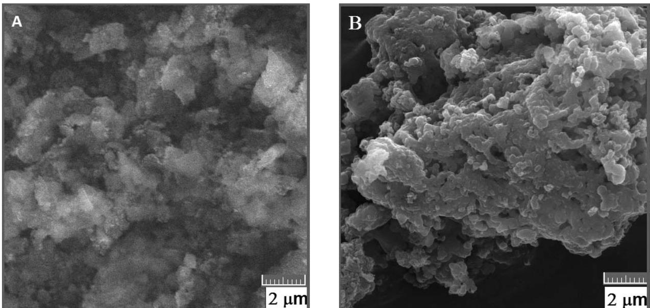
Fig. 4 – SEM micrographs of iri@MCM-41 hybrid sample (A) and MCM-41 support (B).
