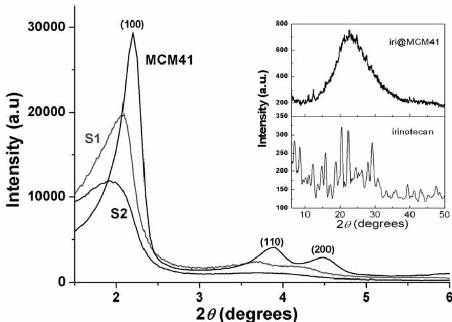
Fig. 1 – Small-angle XRD patterns of the MCM-41-type silica and aluminosilicate supports. Inset-wide-angle XRD of iri@MCM-41 (up) and irinotecan hydrochloride (bottom).
