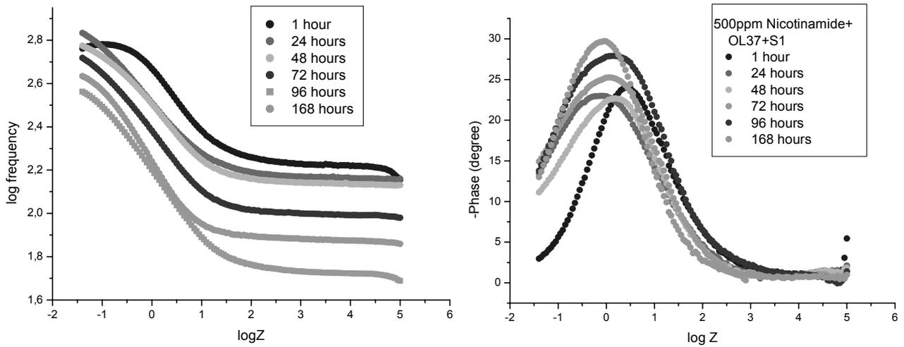
Fig. 9 – The Bode plot for OL37 in S1 with organic inhibitor and at different immersion times.
