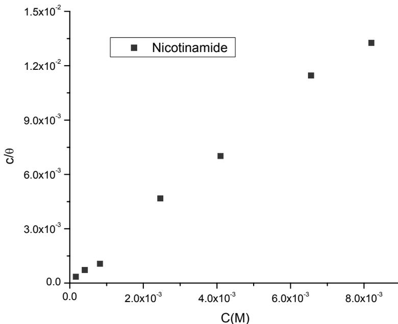
Fig. 5 – Langmuir plot for OL-37+Nicotinamide at different inhibitor concentrations and different immersion times.
