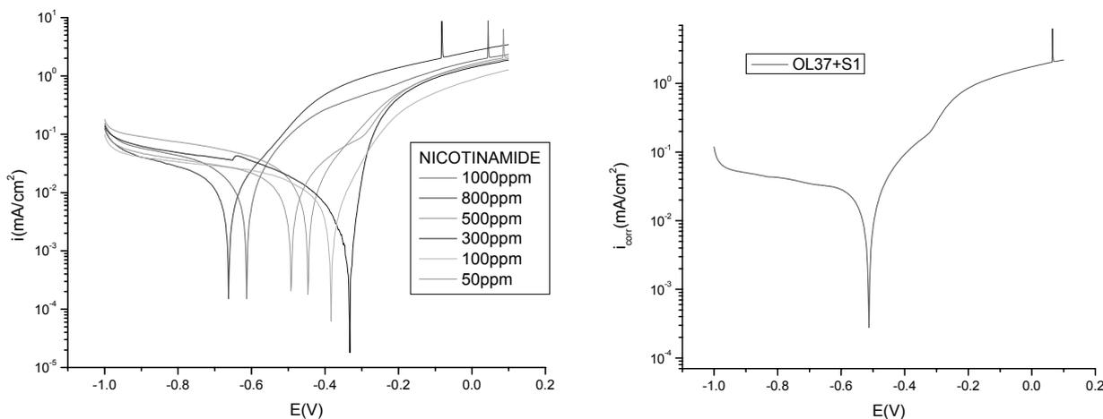
Fig. 1 – The polarization curves of OL 37 carbon steel in cooling water type S1 in presence and absence of Nicotinamide.
