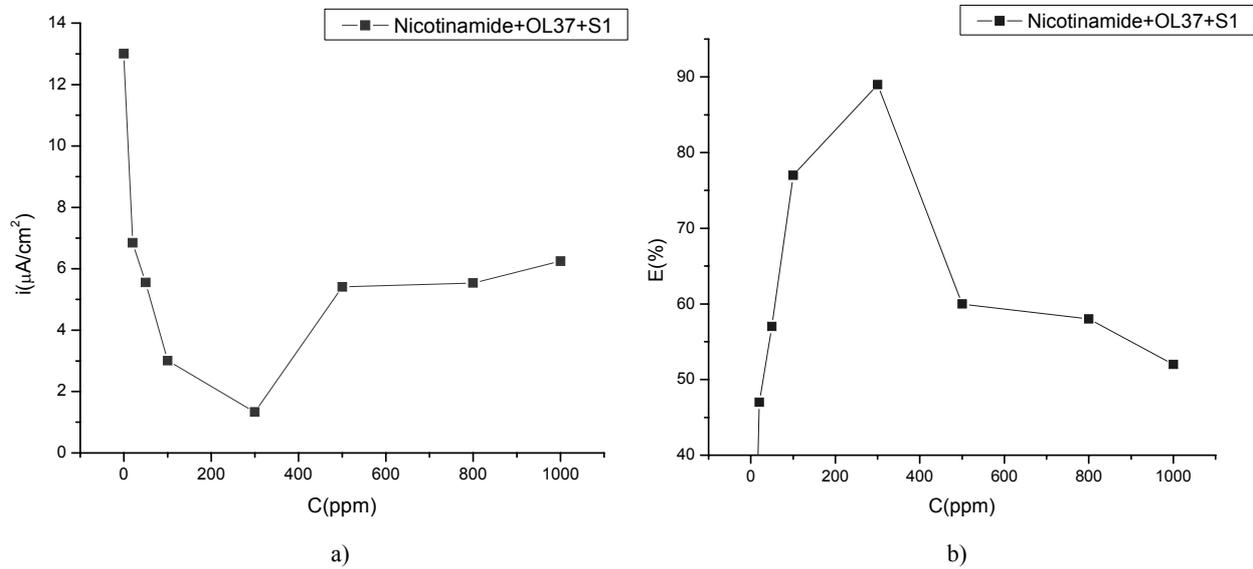
Fig. 3 – The influence of the inhibitor (Nicotinamide) concentration on the corrosion rate of carbon steel OL 37 in cooling water type S<sub>1</sub> (Fig. 3a) and the influence of the inhibitor concentration with efficiency (Fig. 3b) at a temperature of 25<sup>o</sup>C.
