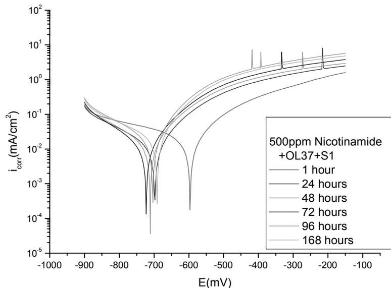
Fig. 2 – The polarization curves of OL 37 carbon steel in cooling water type S1 in presence of 500ppm Nicotinamide at different immersion times.
