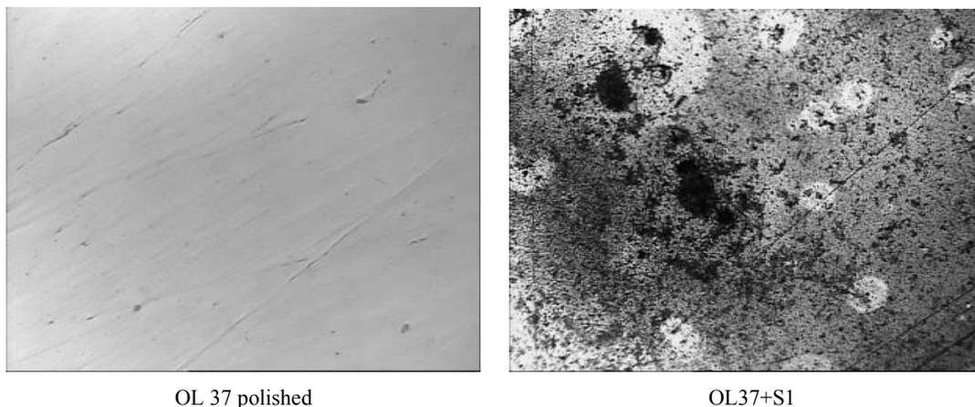
Fig. 12 – Micrographies of the carbon steel in cooling water S1: a) OL 37 polished, b) OL37+S1.
