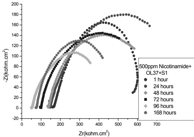
Fig. 8 – The Nyquist plot for OL37 in S1 with organic inhibitor and at different immersion times.
