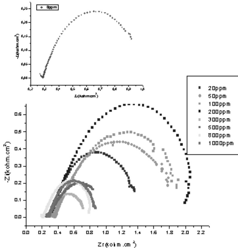
Fig. 6 – The Nyquist plot for OL37 in S1 with and without organic inhibitor.
