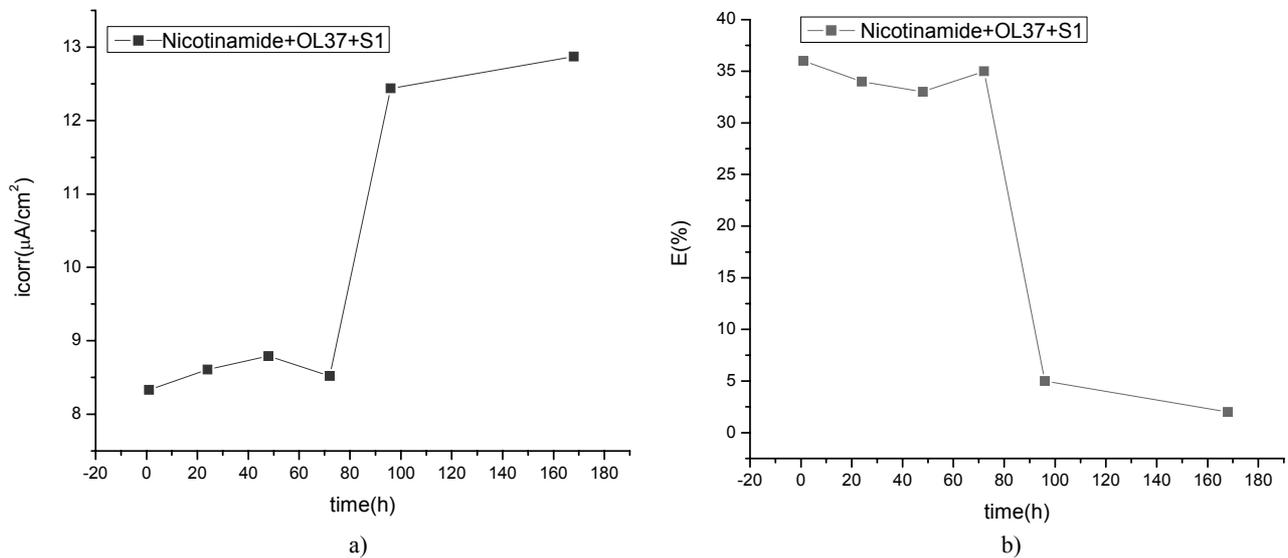
Fig. 4 – The influence of immersion times of the inhibitor (500ppm Nicotinamide) on the corrosion rate and efficiency of carbon steel OL 37 in cooling water type S<sub>1</sub>.
