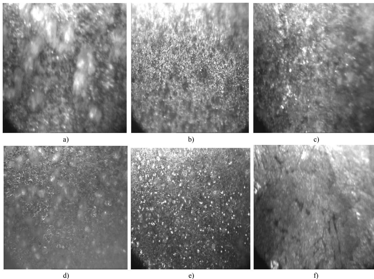
Fig. 13 – Micrographies of the carbon steel in cooling water S1 with organic inhibitor: a) OL37+100ppm Nicotinamide, b) OL37+300ppm Nicotinamide c) OL37+500ppm Nicotinamide d) OL37+800ppm Nicotinamide, e) OL37+500ppm Nicotinamide at 1h immersion time f) OL37+500ppm Nicotinamide at 72 h immersion time.
