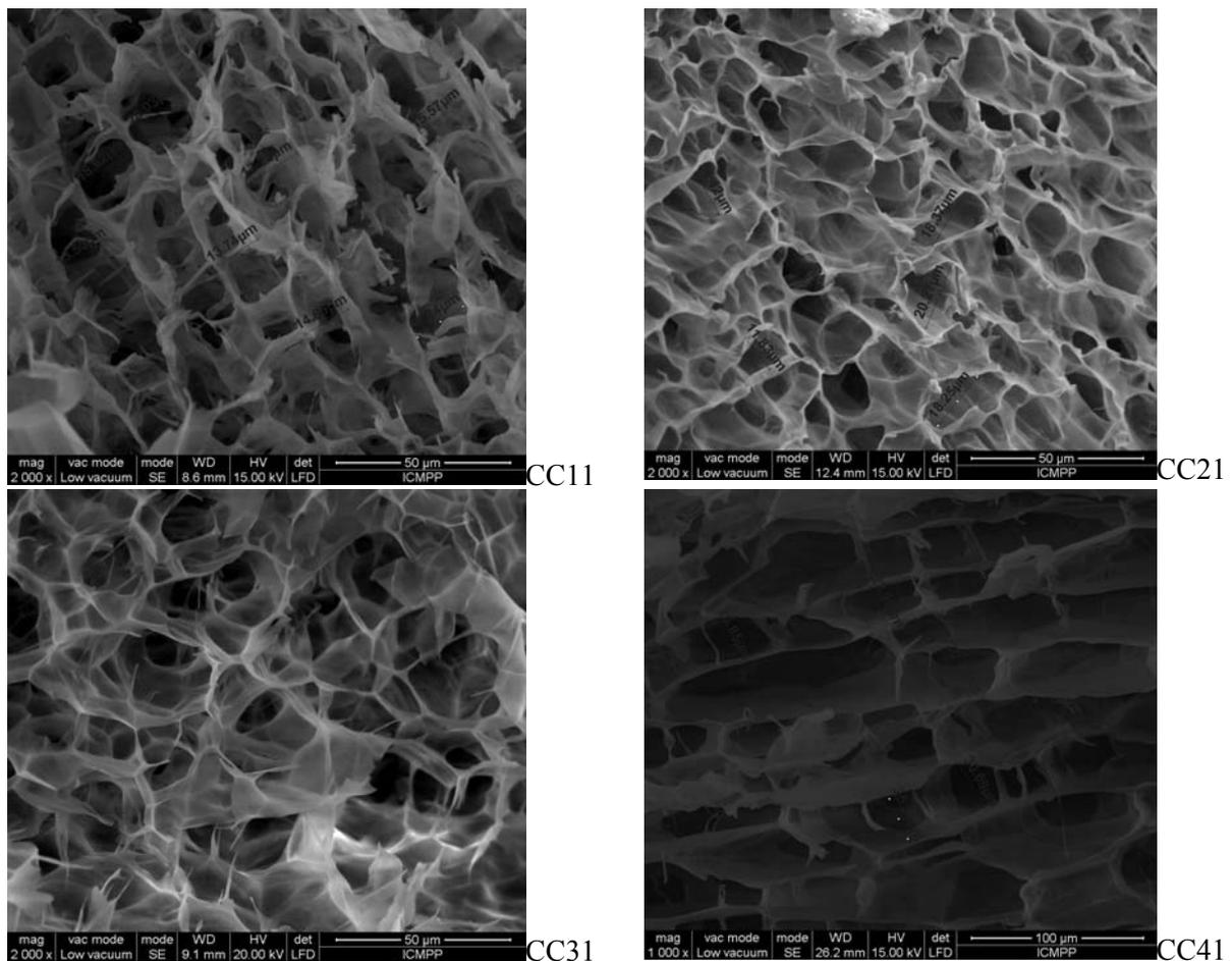
Fig. 6 – SEM microphotographs of the cinnamaldehyde-chitosan hydrogels.
