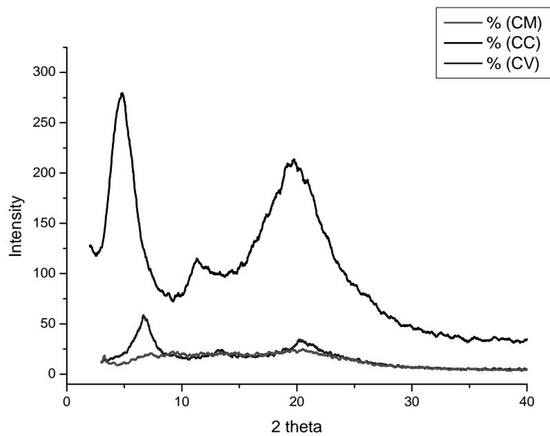
Fig. 5 – XRD pattern of the imino-chitosan derivatives.
