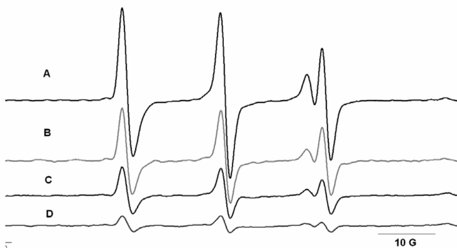
Fig. 6 – EPR spectra of TEMP after mixing with unexposed plant extract A) immediately after mixing TEMP with the extract, B) after 2 minutes, C) after 4 minutes, D) after 8 minutes.
