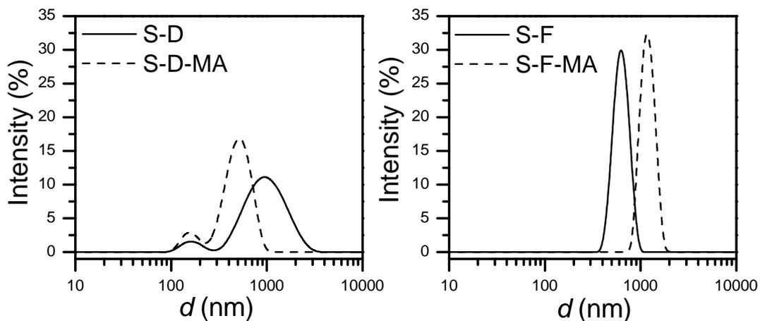
Fig. 3 – Particle size distribution of the designed suspensions prepared with untreated powder (S-D and S-F) and with mechanically treated powder (S-D-MA and S-F-MA).
