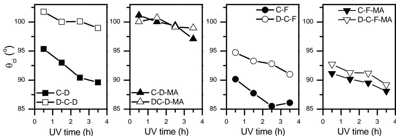
Fig. 7 – Average initial contact angle of studied coatings as function of the UV irradiation time before and after durability testing.
