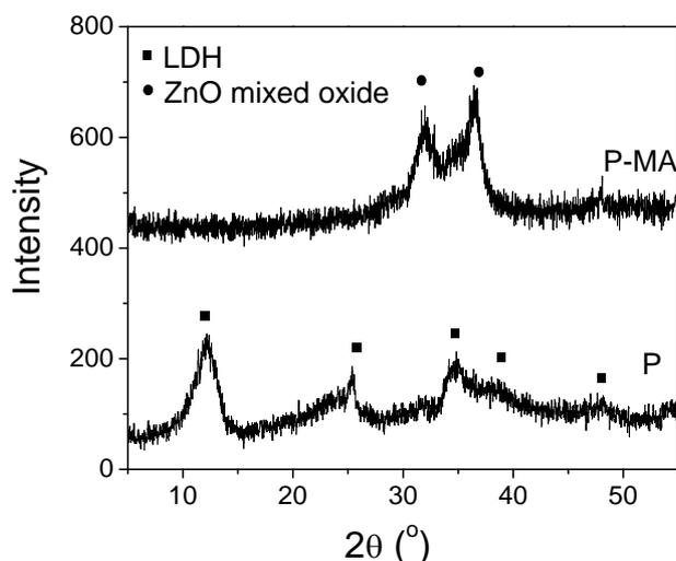
Fig. 1 – XRPD pattern of the as synthesized powder (P) and the mechanically treated powder (P-MA).
