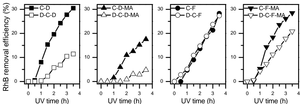
Fig. 6 – RhB removal efficiency of studied coatings before and after durability testing.
