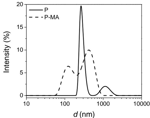
Fig. 2 – Particle size distribution of the as synthesized powder (P) and of the mechanically treated powder (P-MA).
