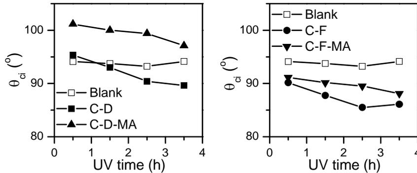
Fig. 5 – Average initial contact angle of all studied coatings as function of the UV irradiation time.
