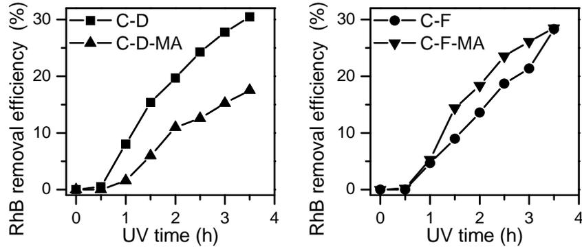
Fig. 4 – RhB removal efficiency of the studied coatings.
