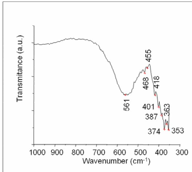
Fig. 3 – IR spectra for Ni ferrite thermally treated at 900°C.
