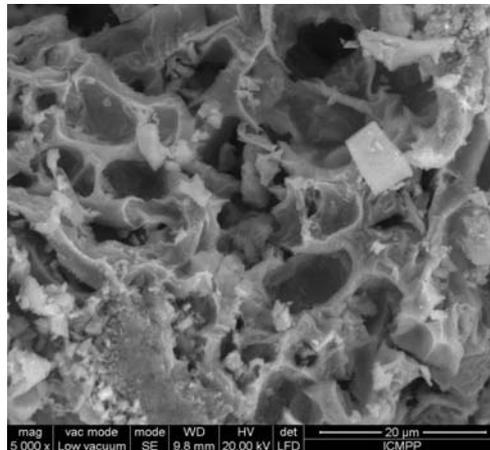
Fig. 5 – SEM micrography for Ni ferrite thermally treated at 900°C.
