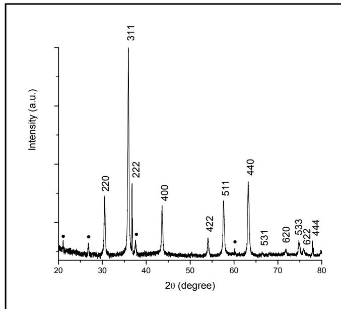
Fig. 4 – XRD pattern for Ni ferrite thermally treated at 900°C.
