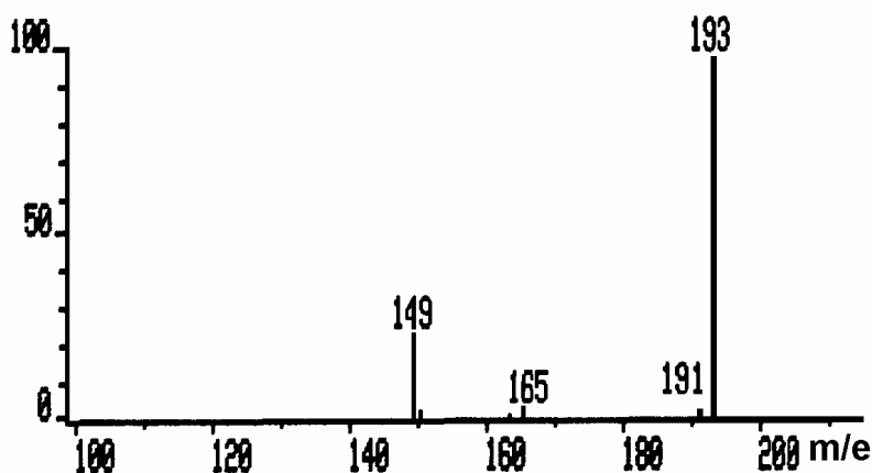
Fig. 2 – The daughter ions of the primary fragmentation ion with m/e 193 obtained by the B/E linked scan.
