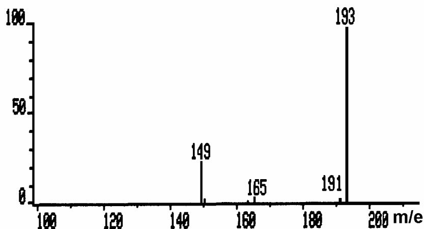
Fig. 4 – The TEOS fragmentation ions which eliminate ethylene obtained by the B/E(1-E)^{1/2} linked scan.
