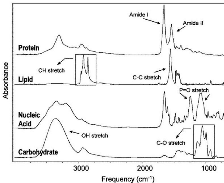
Fig. 3 – Various cellular components have dramatically different IR spectra as demonstrated by IR spectra of (A) a lipid (palmitic acid), (B) a protein (myoglobin), (C) a poly-nucleic acid, and (D) a carbohydrate (sucrose).
