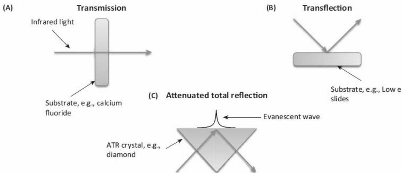
Fig. 4 – Examples of Fourier transform infrared sampling methods for: (A) transmission mode experiments; (B) transflection mode experiments; (C) attenuated total reflection (ATR) mode experiments.
