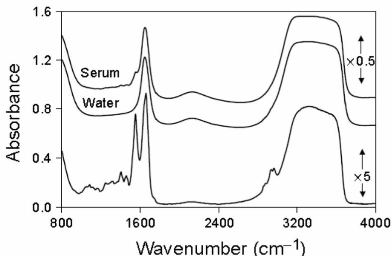
Fig. 1 – MIR absorption spectra of serum and water, collected with an optical path of 6  $\mu\text{m}$ . The lower spectrum is the difference, water spectrum subtracted from the serum one.
