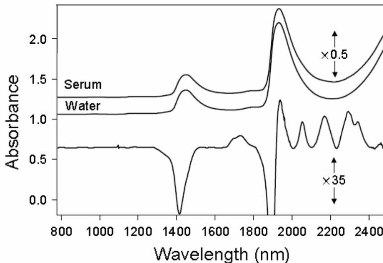
Fig. 2 – NIR absorption spectra of serum and water, collected with an optical path of 0.5  $\mu\text{m}$ . The lower spectrum is the difference, water spectrum subtracted from the serum one.
