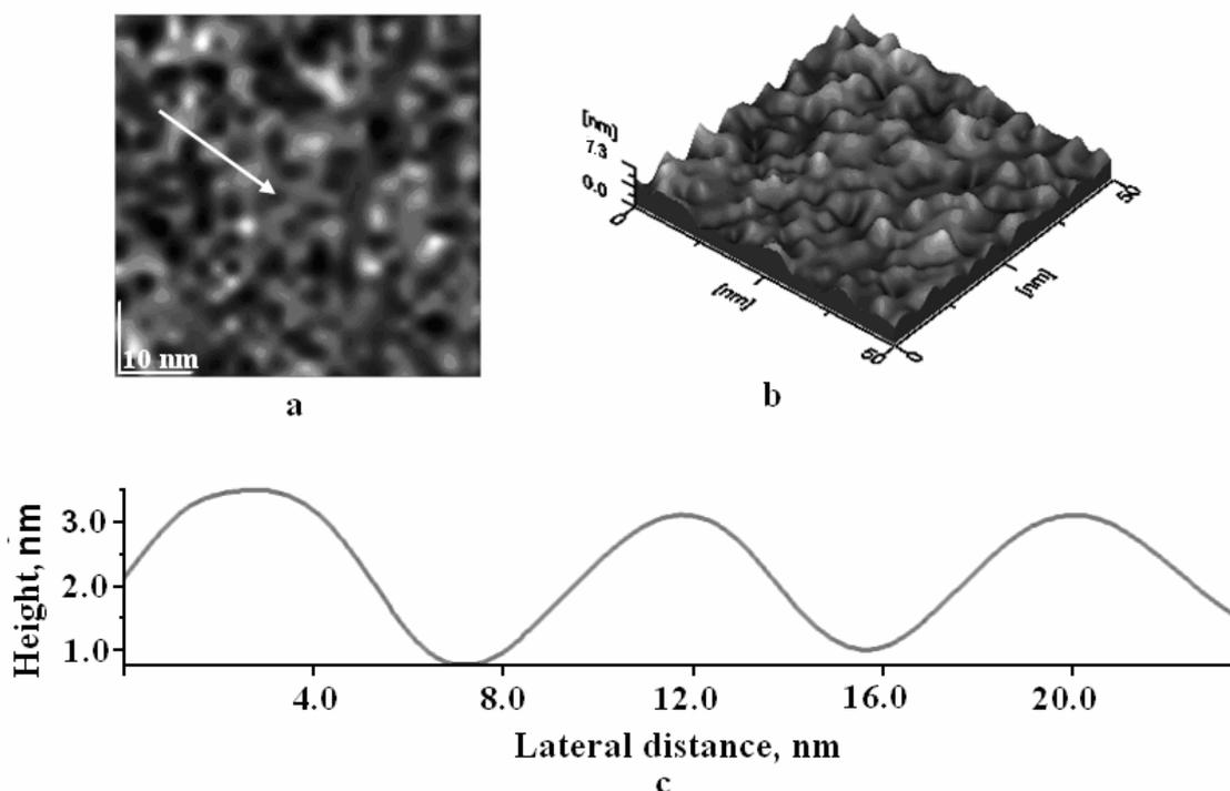
Fig. 3 – AFM images of GNPs assembled on glass: (a) 2D- topography; (b) 3D – topography; (c) profile of the cross section along the arrow in panel a; scanned area 50 nm x 50 nm.
