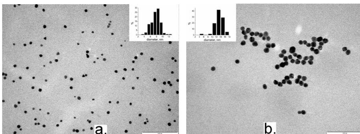
Fig. 2 – TEM images of GNPs (a) and SNPs (b). The bars in TEM images correspond to 100 nm. Inserts are the histograms of size distribution.
