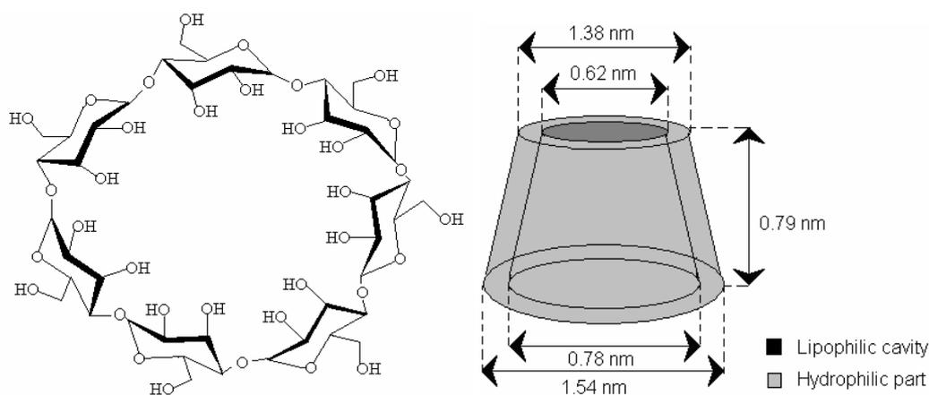
Scheme 1 – Structure and geometric sizes of  $\beta$ -cyclodextrin.
