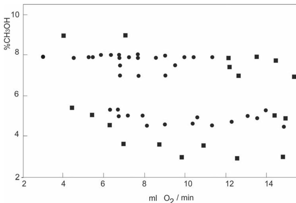
Fig. 1 – Experimental area for methanol concentration and oxygen flow rate, where thermal oscillations may be detected during methanol oxidation at 80 C on 20 mg palladium catalyst (● oscillatory regime; ■ non-oscillatory regime).
