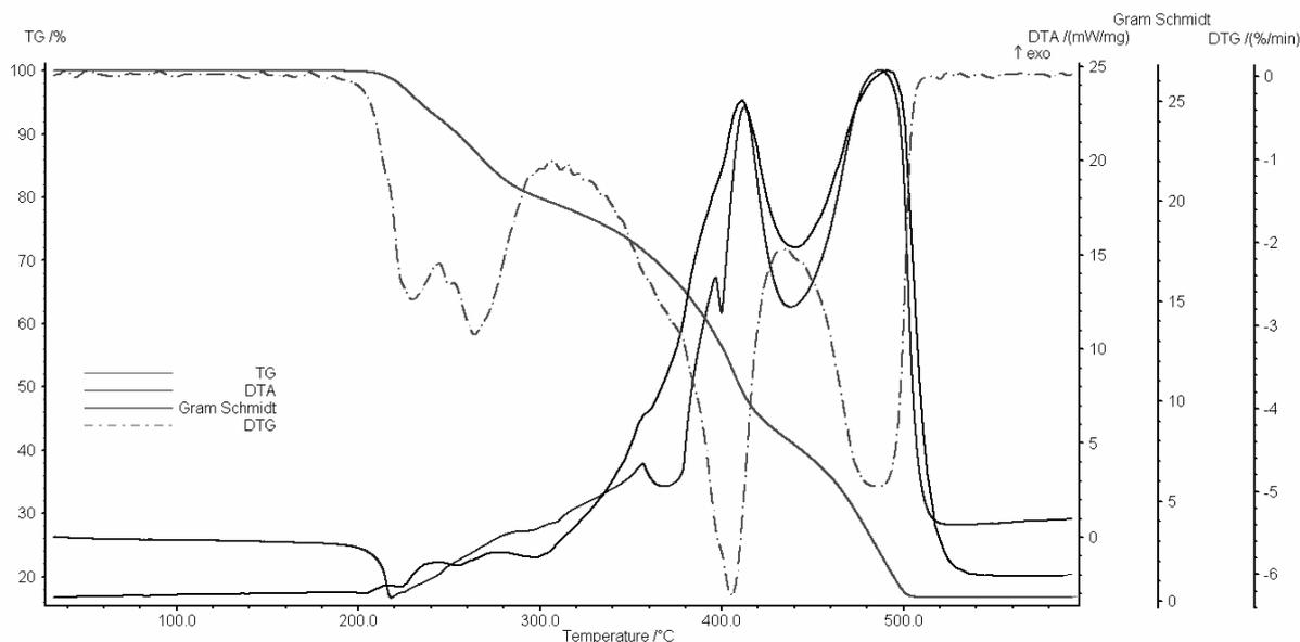
Fig. 4 – TG, DTG, DTA and Gram Schmidt curves for compound 1.
