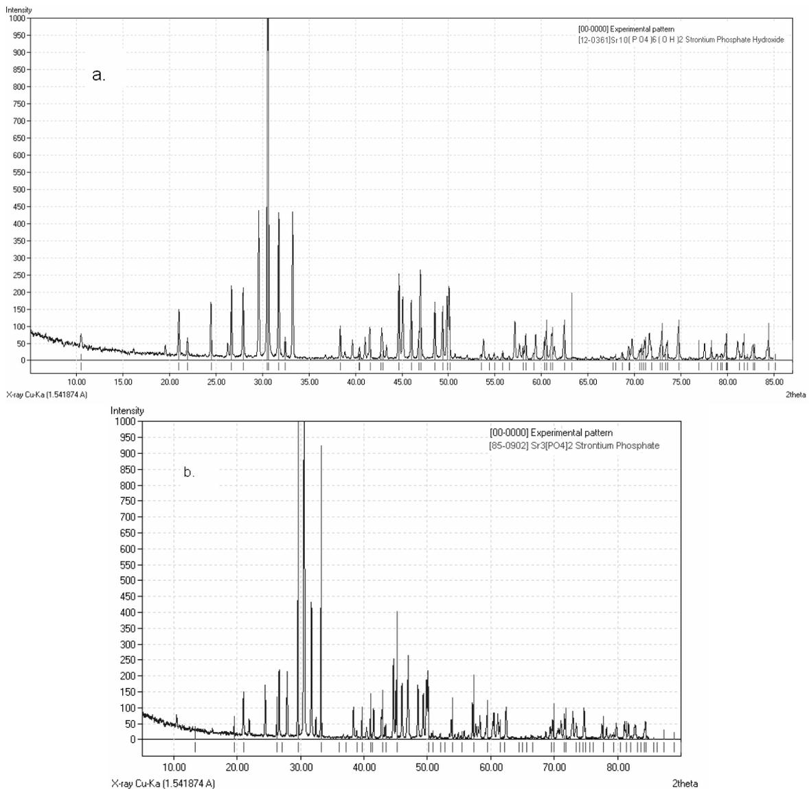
Fig. 1 – XRD pattern for the SrHAP nanopowder compared with PDF for Sr<sub>10</sub>(PO<sub>4</sub>)<sub>6</sub>(OH)<sub>2</sub> (a) and for Sr<sub>3</sub>(PO<sub>4</sub>)<sub>2</sub> (b).
