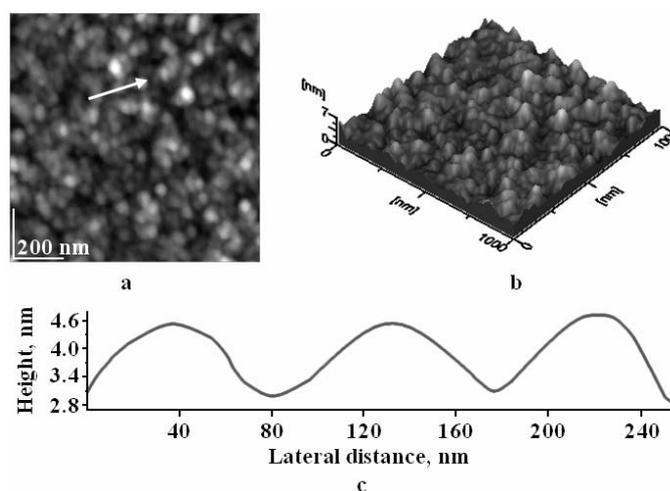
Fig. 4 – HAP-5%Sr adsorbed on glass for 30 s from aqueous dispersion: (a) 2D-topographic image; (b) 3D-topographic image; (c) cross section profile along the arrow in panel (a); scanned area:  $1 \mu\text{m} \times 1 \mu\text{m}$ ; average particle size  $62 \pm 5$  nm.
