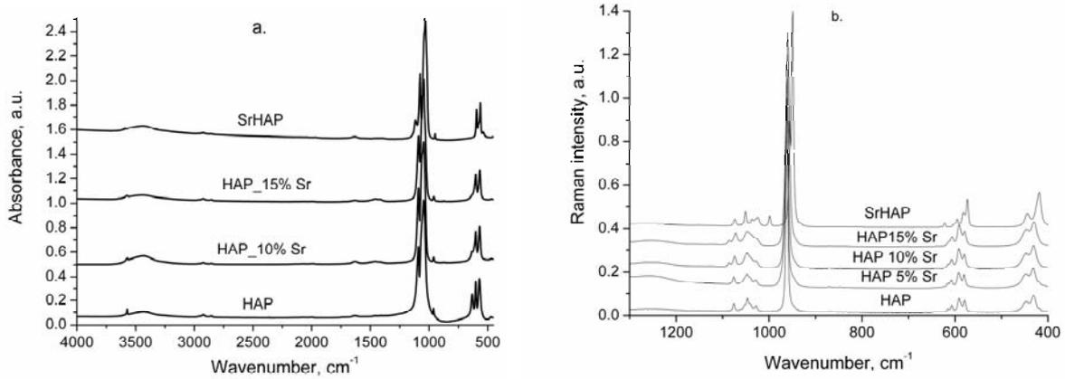
Fig. 2 – Normalized FTIR spectra (a) and Raman spectra (b) of HAP and Sr-substituted HAPs.
