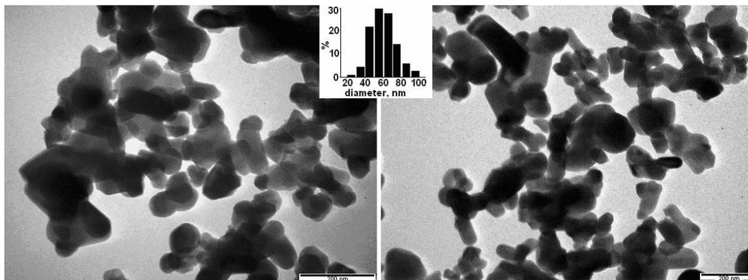
Fig. 3 – TEM images for HAP-15% Sr and histogram of size distribution; bars length: 200 nm; average diameter of the particles:  $\bar{d} = 69 \pm 13$  nm.
